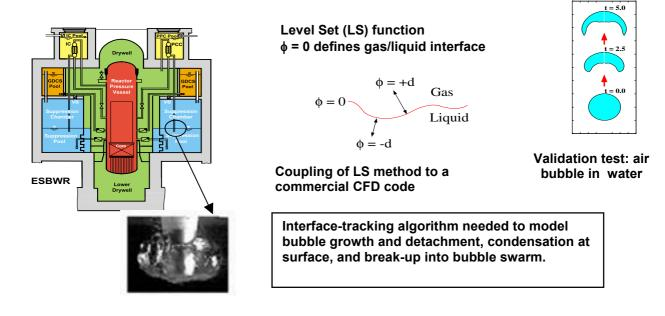
FIG. 13. CFD modelling of gas/liquid interfaces.
