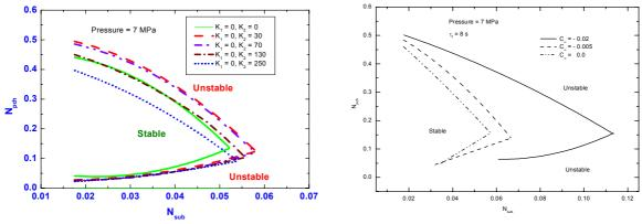
FIG. 14. Effect of inlet orificing on OPO.
