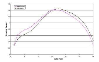
FIG. 25. Steady state mean power axial distribution.
