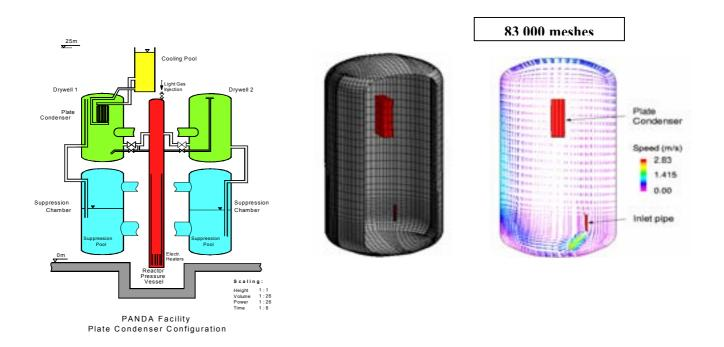
FIG. 11. CFD simulation of plate condenser.
