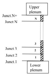
FIG. 10. Boiling channel discretization.
