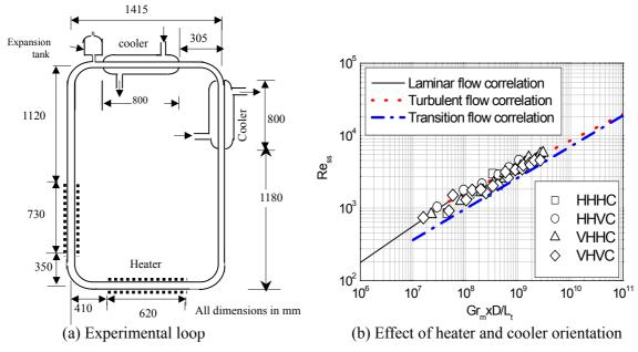
FIG.4. Effect of heater and cooler orientation on steady state NC [8].
