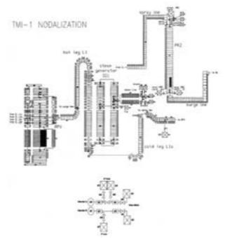
FIG. 2. Sketch of the nodalisation for the TMI-1 MSLB benchmark (entire system).
