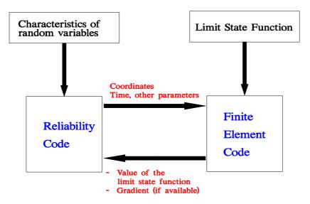
FIG. 4.5. Direct coupling between reliability code and T-H code.
