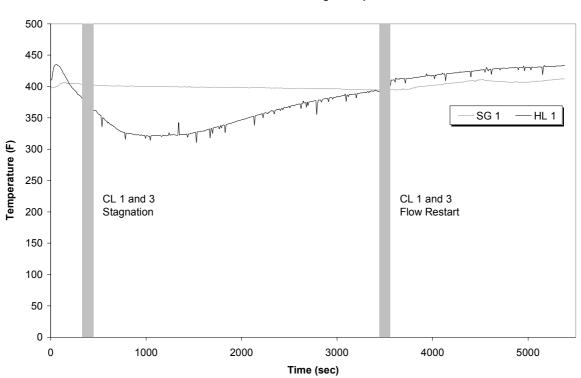
Steam Generator 1 vs. Hot Leg 1 Temperature
