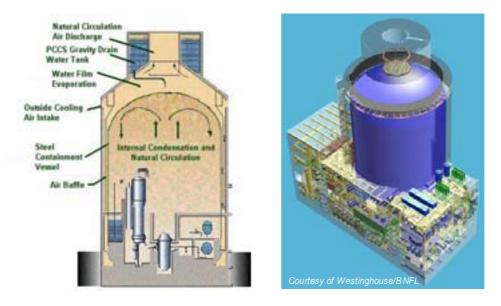
FIG. 6. Containment and passive containment cooling system (PCCS).
