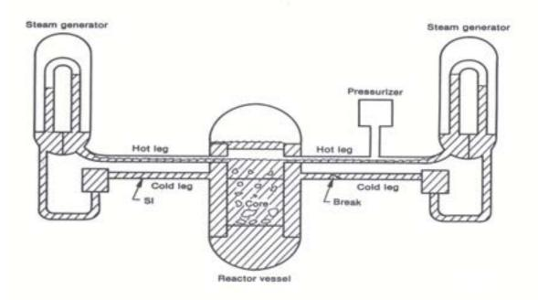
FIG. 2. Formation of a continuous vapor phase at the top of the steam generator U-tube and vessel during a small break LOCA in PWR..
