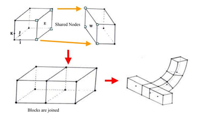
FIG. 3. Hexahedral cells used to build the problem geometry.
