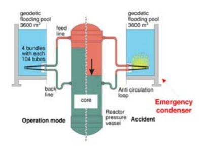
FIG. 4. SWR-1000 emergency condenser.
