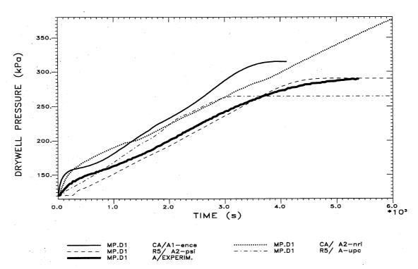
FIG. 8. Drywell pressure RELAP5/Mod3 and CATHARE code calculations compared to experimental data for Phase A of ISP-42.
