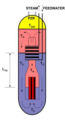
FIG. 9. Hot and cold regions of single-phase natural circulation flow within an integral reactor.
