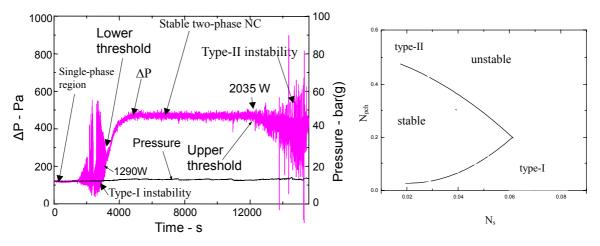
FIG. 1a. Typical low power and high power unstable zones for two-phase NC flow.
