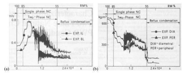
FIG. 12. Velocites (a) and density (b) in the two loops of the facility (IL - intact loop - designates a lumped loop, representing three loops of the plant, while BL - broken loop - represents a single loop).
