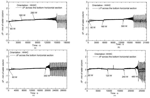
FIG. 12. Instability development by the oscillation growth mechanism.
