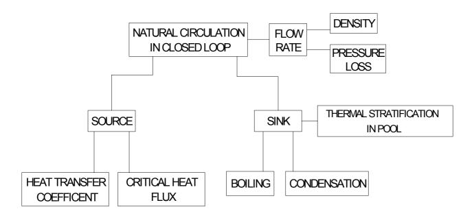
FIG. 6. Important phenomena/ parameters relevant to natural circulation in closed loop.
