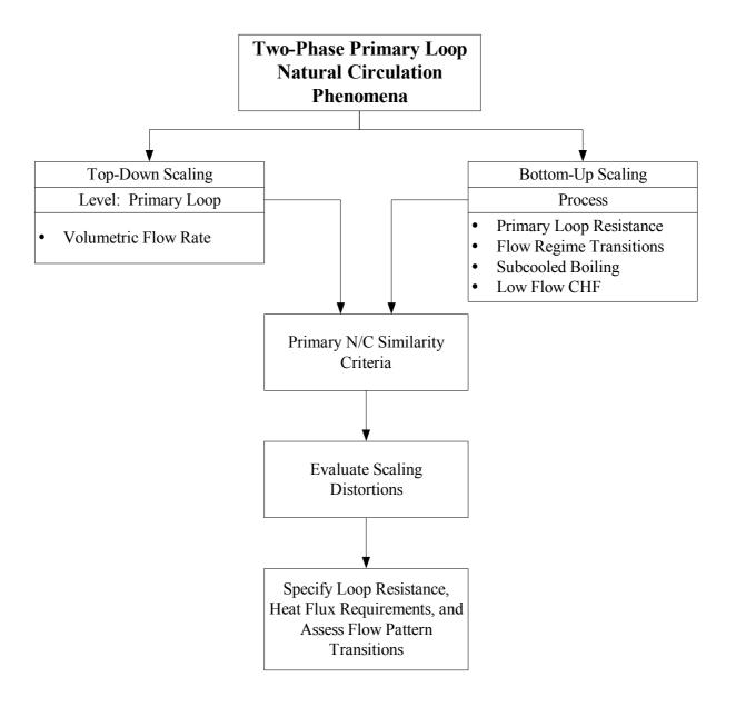
FIG. 9. Scaling analysis flow diagram for two-phase natural circulation.
