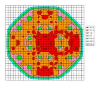
FIG. 23. Steady state 2D flux core distribution.
