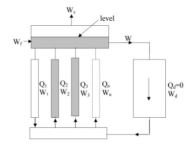
FIG. A2.1. A NCS with n parallel vertical unequally heated channels.
