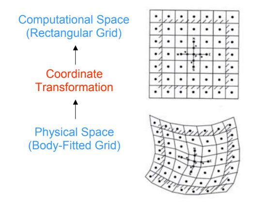
FIG. 5. Example of coordinate transformation process.
