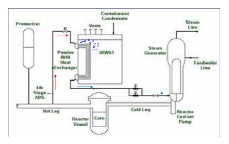
FIG. 4. Passive residual heat removal (PRHR) system.
