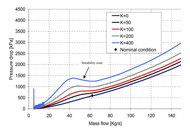
FIG. 2. Calculation of the static SG characteristics with Relap5 code; effect of the energy loss coefficient (in two phase zone) on the pressure drop characteristic.
