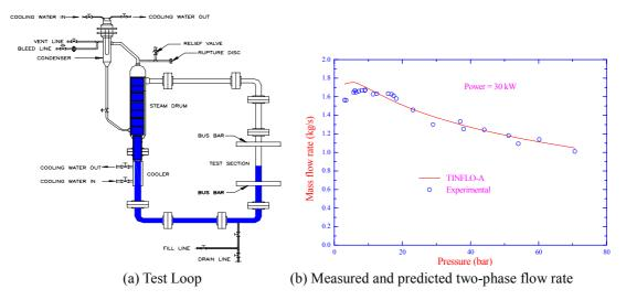
FIG. 11. Effect of pressure on two-phase NC flow rate.
