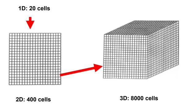
FIG. 2. The rapid growth in the number of mesh cells in going from 1-D to 3-D problems.
