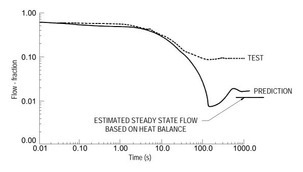
FIG. 6. Variation of flow rate for test at 1.991%FP.
