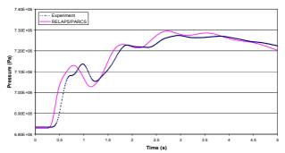
FIG. 26. Core pressure wave evolution.
