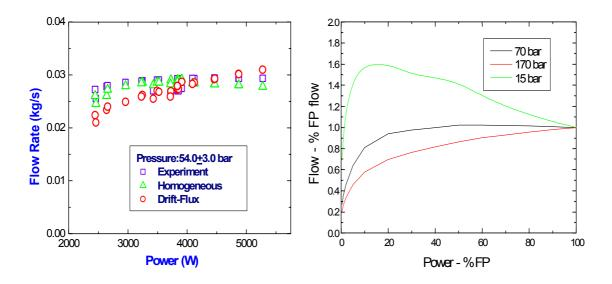
*FIG. 12a. Measured and predicted flow rates* howing the effect of power.
