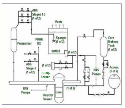
FIG. 5. Passive safety injection and sump recirculation.
