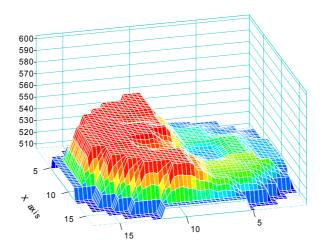
FIG. 7a. Core outlet coolant temperature in Phase 2 scenario B r5qc calculation.
