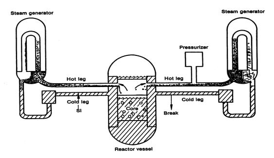
FIG. 3. Initiation of core uncovery during a small break LOCA in PWR..
