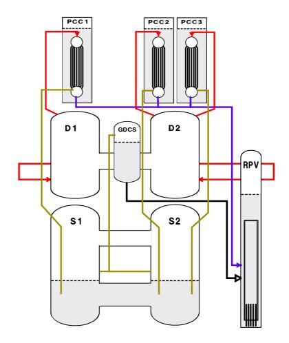
FIG. 5. ISP-42 Phase A: Passive containment cooling system start-up.
