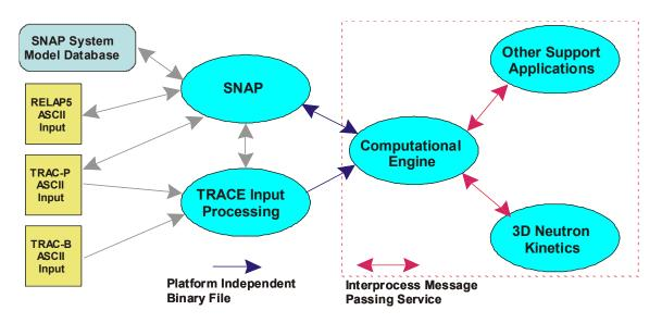
FIG. 4. TRACE /SNAP environment architecture [10].
