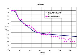
FIG. 36 Transient pressurizer level.
