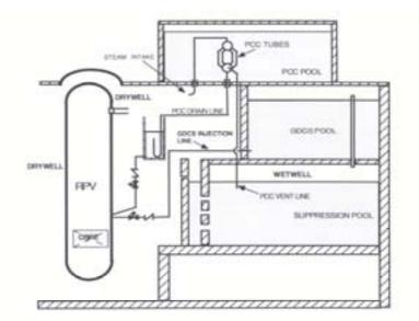
FIG. 6. The ESBWR passive containment cooling system condenses containment steam and vents the non-condensable to the suppression pool.
