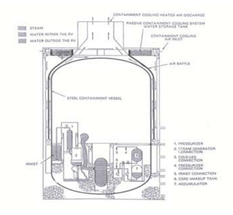
FIG. 6. Passive containment cooling for the AP600/AP1000 design.
