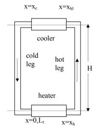
FIG. A1.1 : A uniform diameter rectangular loop
