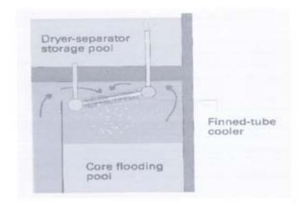
FIG. 8. Containment cooling condenser for SWR1000.
