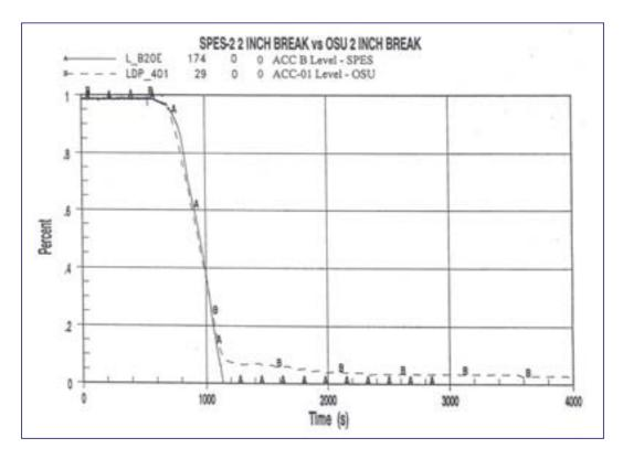
FIG. 15. Comparison of SPES-2 and APEX-600 two-inch SBLOCA accumulator liquid level histories.
