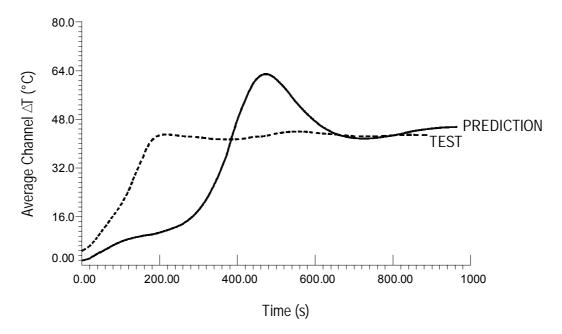
FIG. 9. Variation of average channel delta-T for test at 1.991%FP.
