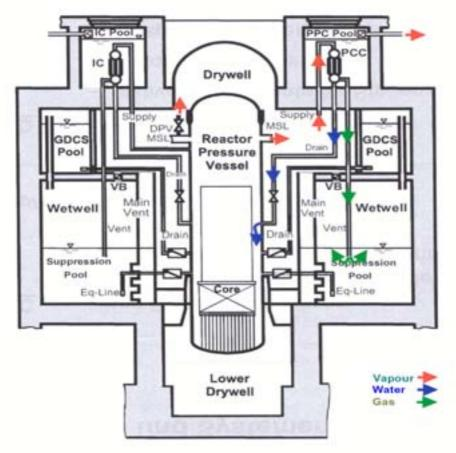
FIG. 4. The ESBWR design and passive safety systems.
