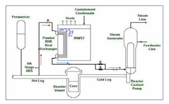
FIG. 1. AP1000 passive residual heat removal systems (PRHR).
