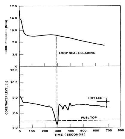
FIG. 5. Typical transients of the primary system pressure and reactor vessel water level following a small break LOCA at the cold leg in a PWR.
