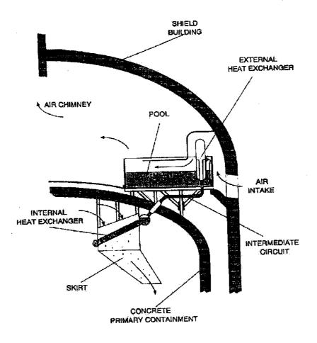
FIG. 7. Double concrete containment passive cooling system proposed as an alternative to the AP600 external wall-cooling concept.
