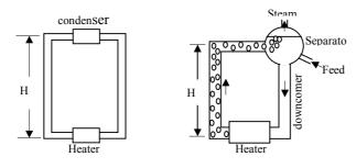
(a) Loop relevant to PWRs (b) Loop relevant to BWRs
