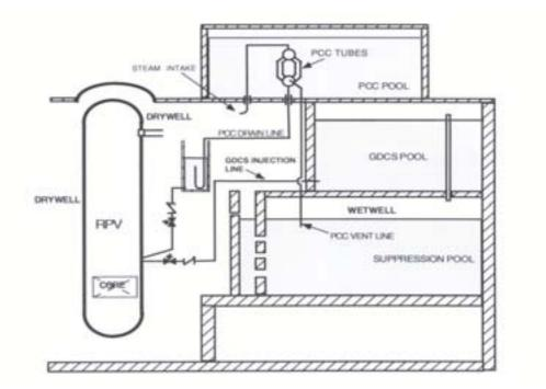
FIG. 9. The ESBWR passive containment cooling system condenses containment steam and vents the non-condensable to the suppression pool.
