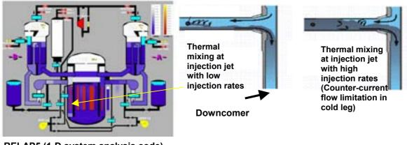
RELAP5 (1-D system analysis code) model of a small break LOCA
