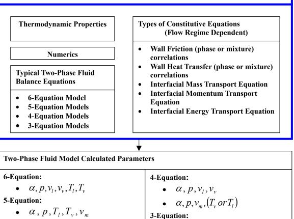
FIG. 2. Types of two-phase flow models used in nuclear reactor safety analyses.
