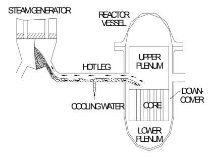
FIG. 15 Countercurrent flow of steam and cooling water in hot leg of PWR.
