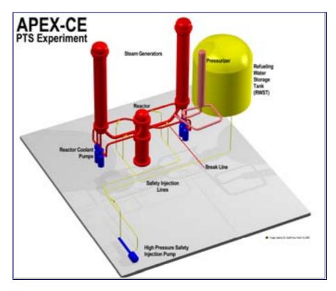
FIG. 1. Schematic of the APEX-CE test facility.
