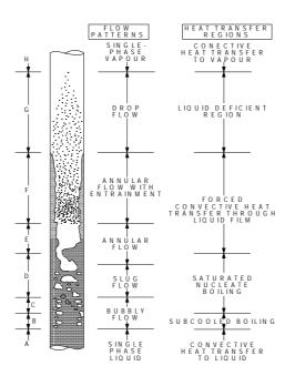
FIG.8. Regions of heat transfer in convective boiling.
