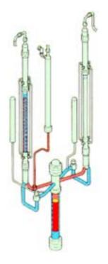
FIG. 15. Schematic of JAERI's large scale test facility (LSTF).
