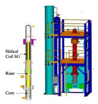
FIG. 18. Schematic of the MASLWR test facility to simulate integral type LWRs.
