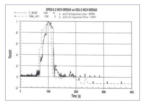
FIG. 16. Comparison of SPES-2 and APEX-600 two-inch accumulator flow histories.
