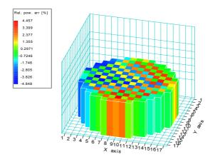
FIG. 21. Relative error in  $f_{xy}$  power peaking factor at t = 60 s calculated by Parcs and Quabbox based coupled codes (direct coupling).
