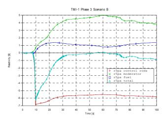
FIG. 16. Reactivity components calculated by Relap5/mod3.2 gamma / Parcs coupled codes.
