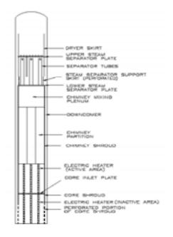
FIG. 19. Schematic of the PUMA test facility to simulate advanced BWRs.
