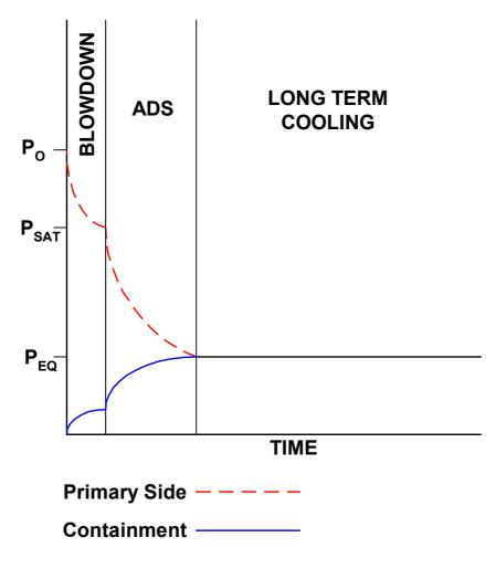
FIG. A.3. Illustration of transient phases for a MASLWR SBLOCA.
