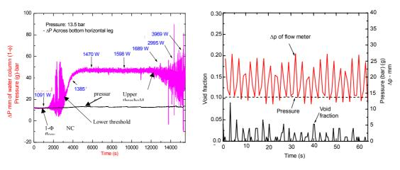
FIG. 26. Typical experimental stability map at 13.7 bar.
