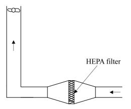
FIG. 2. Schematic of the ventilation system.
