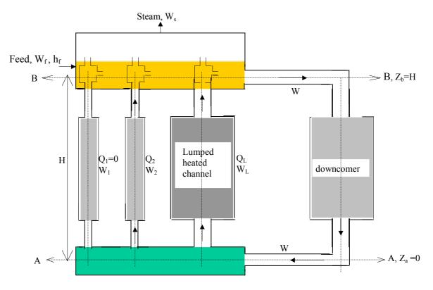
FIG. A2.3. Two-phase parallel channel system.
