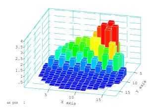
FIG. 20. Relative radial power distribution at t = 60 s calculated by Relap5/mod3.2 gamma /Parcs based coupled code (direct coupling).
