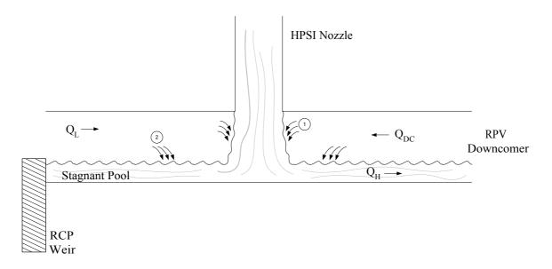
FIG. 13. Thermally stratified conditions for the top-entry HPI..
