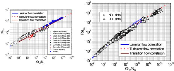
FIG. .8. NDL data neglecting local losses. FIG. .9. All single-phase NC data neglecting local losses.
