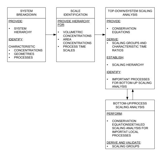
FIG. 4. Flow diagram for the hierarchical, two-tiered scaling analysis. [1].
