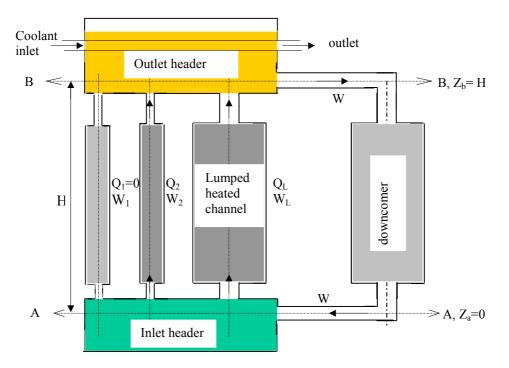
FIG. A2.2. Single-phase parallel channel system.
