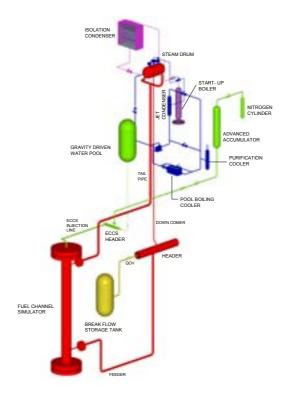
FIG. 13. Schematic of the BARC integral test loop to simulate the AHWR.
