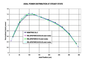
FIG.34. Steady \_state mean axial power profile.
