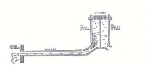
FIG. 7. Schematic of liquid distribution during reflux condensation in PWRs.
