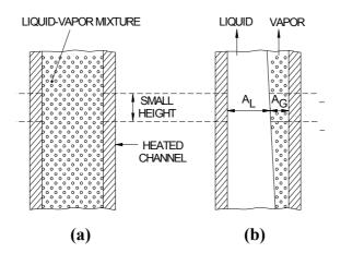
FIG. 7. Two phase flow in a vertical heated channel.
