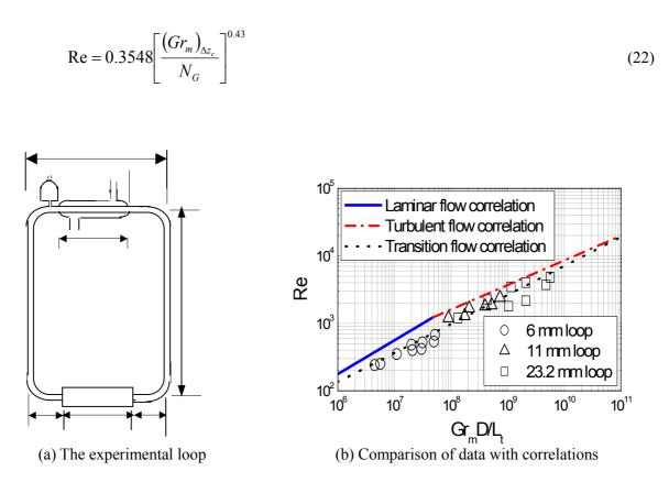
FIG.3. Effect of loop diameter on steady state NC [7].
