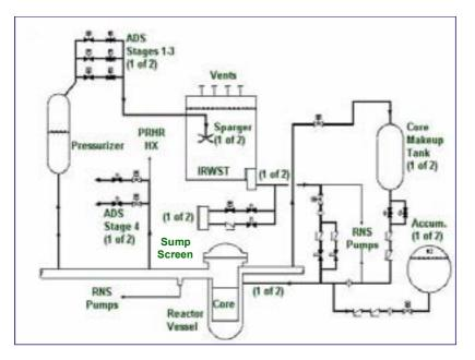
FIG. 2. Schematic of the AP1000 passive safety systems including the CMTs and sump recirculation system.
