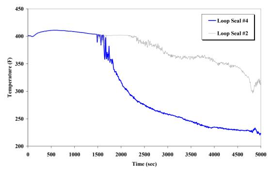
FIG. 6. Asymmetric loop seal cooling (OSU-CE-0008).
