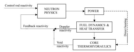
FIG. 16. The BWR feedback loop.
