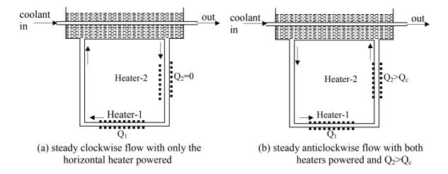
FIG. 4. Effect of flow direction on the instability.
