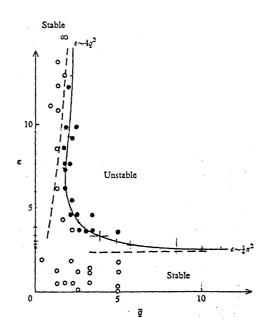
FIG. 7. The (pen and paper) curve which separates the stable from the unstable region. Remember that  $\varepsilon = RL/(2k\Delta s)$ . So epsilon increases when the friction increases, and decreases when the quantity of heat transferred at the heat sink and source increases.  $\overline{q}$  indicates the flow rate of the steady state solution. The dots indicate numerical experiments. A solid dot means the numerical solution turned out to be unstable, an open circle indicates a stable solution.
