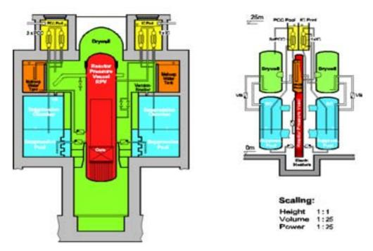
FIG. 3. SBWR versus PANDA test facilty.
