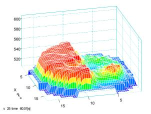
FIG. 7b. Core outlet coolant temperature in Phase 2 scenario B r5qcv calculation.
