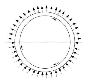
FIG. 5. Toroidal loop with bottom half heated and top half cooled.
