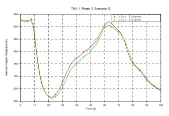
FIG. 18. Maximum Doppler temperature calculated by Parcs and Quabbox based coupled codes (direct coupling).
