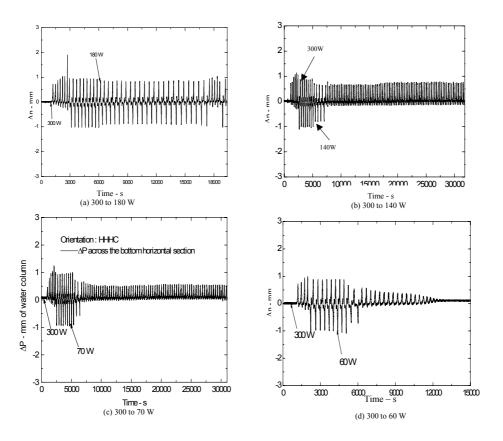
FIG. 15. Stability threshold for power reduction from an unstable state.
