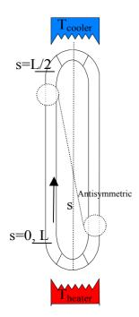
FIG. 5. A simple closed loop with a heater at the bottom and a heat sink at the top. It is filled with liquid in subcooled conditions.
