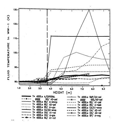
FIG. 10. Measured and predicted axial temperature distribution in wetwell-1 at 4000s for Phase A of ISP-42.
