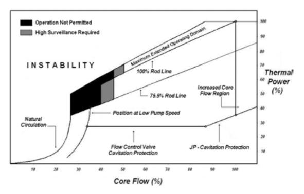
FIG. 1. Instability region in the power-flow map for the Leibstadt NPP.
