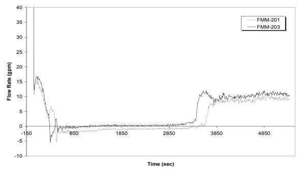
FIG. 4. Illustration of loss of natural circulation flow during a main steam line break simulation and recovery (OSU-CE-0012).
