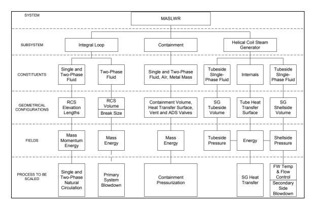
FIG. 6. MASLWR system breakdown into components, geometries, fields and processes.
