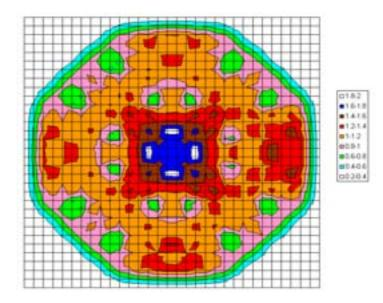
FIG. 31. Steady state mean 2D core power distribution for single channel model.
