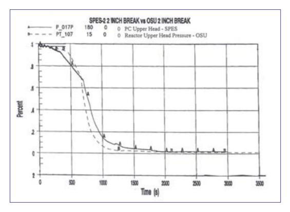
FIG. 12. Comparison of SPES-2 and APEX-600 two-inch SBLOCA pressure histories.
