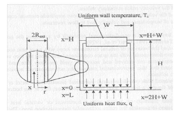
FIG. 3. The natural circulation loop investigated by [1]. Two spatial (x,r) and one time coordinate (t) were used. A uniform heat flux was imposed. The materials and therefore the heat capacities for the piping was varied. The results showed that the heat capacity of the piping has a considerable influence on the behavior of the system.
