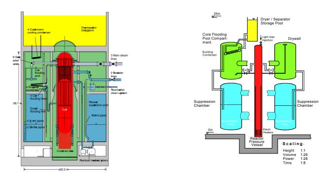
FIG. 4. SWR 1000 versus PANDA test facility.
