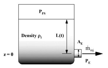
FIG. 7. Schematic for a passive safety system tank.
