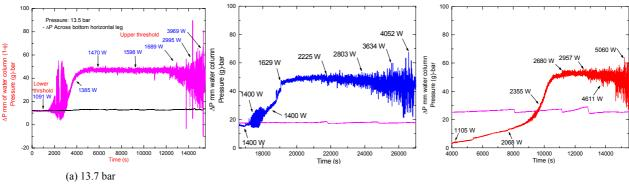
FIG.31. The upper threshold of instability at different pressures.
