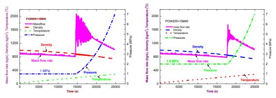
FIG. 20. Heat up procedure with one time pressurization.
