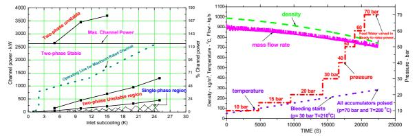
FIG. 18. Stability map for OPO in AHWR.
