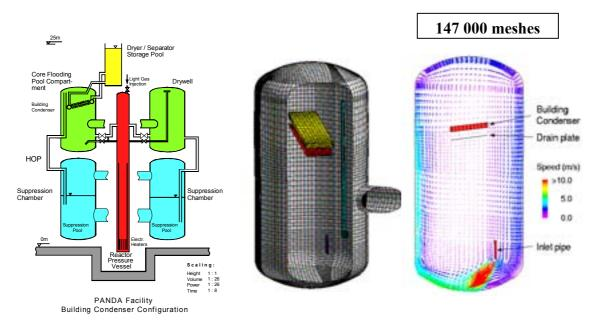
FIG. 10. CFD simulation of building condenser.
