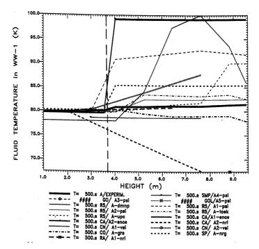
FIG. 9. Measured and predicted axial temperature distribution in wetwell-1 at 500s for Phase A of ISP-42.
