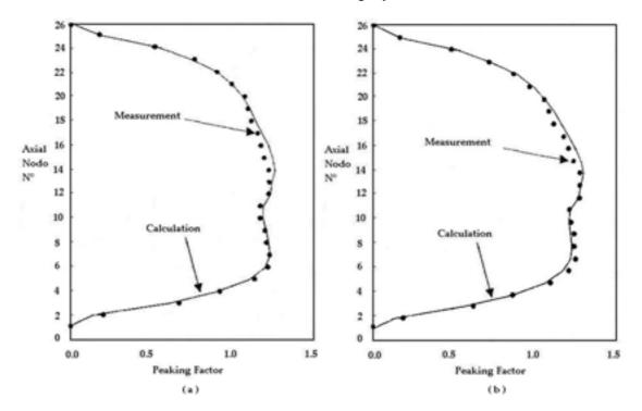
FIG. 7. Correlation between calculated and measured axial power profiles:
