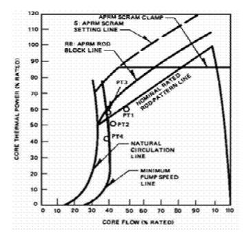
FIG.3 Peach Bottom-2 low-flow test conditions.
