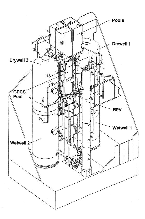
FIG. 1. 3-D View of the PANDA test facility.
