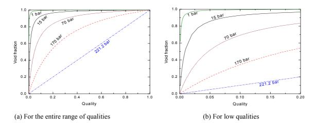
FIG. 13. Effect of pressure on the void fraction.
