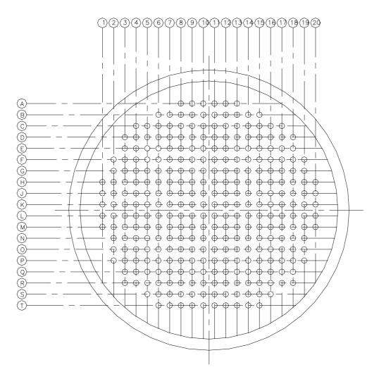
FIG. 2. Core configuration.
