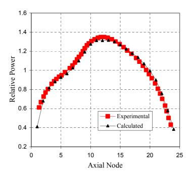
FIG. 4. Steady State mean power axial distribution.
