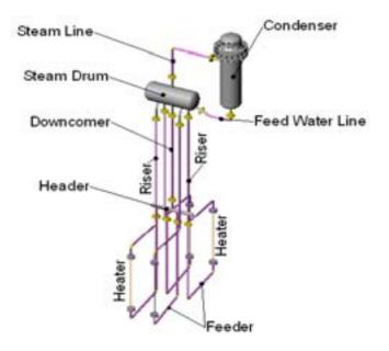
FIG. 14. Schematic of BARC Parallel Channel Loop (PCL)
