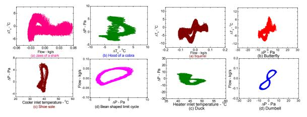
FIG. 19. Parametric effect on the phase plots for UDP at 140 W.
