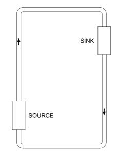
FIG. 8. A Rectangular closed natural circulation loop.
