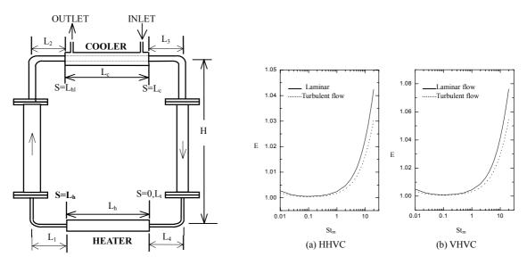
FIG. 1. NCL with horizontal heater and cooler.
