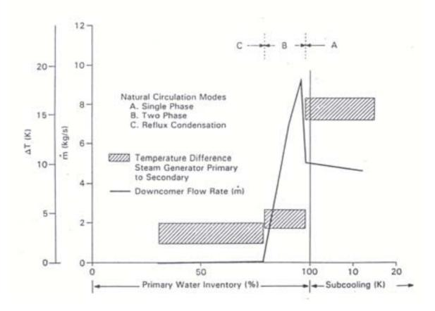
FIG. 8. Mass flow rates and primary to secondary temperature differences as functions of primary mass inventory for PKL test facility.
