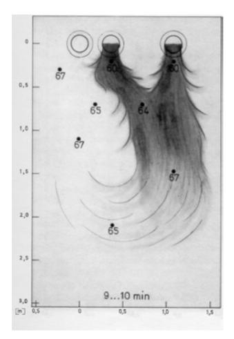
FIG. 20. Downcomer plume interactions as observed in IVO 2/5 scale transparent test loop (IVO Mixing Test #115).
