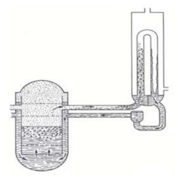
FIG. 4. Liquid inventory trapped outside of the reactor vessel due to a loop seal.
