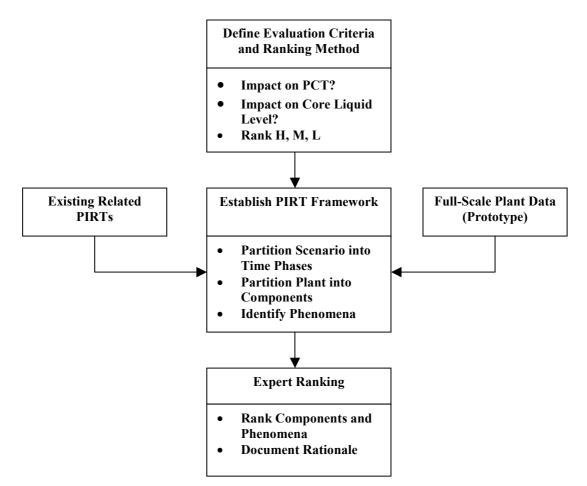
FIG. 3. Process used to develop a "Phenomena Identification and Ranking Table" (PIRT).
