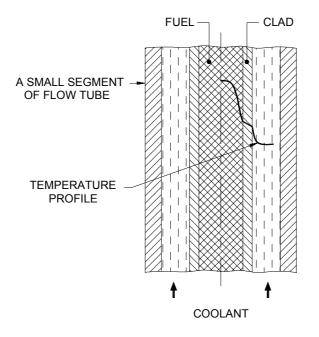
FIG. 2. Radial temperature distribution in fuel and coolant.
