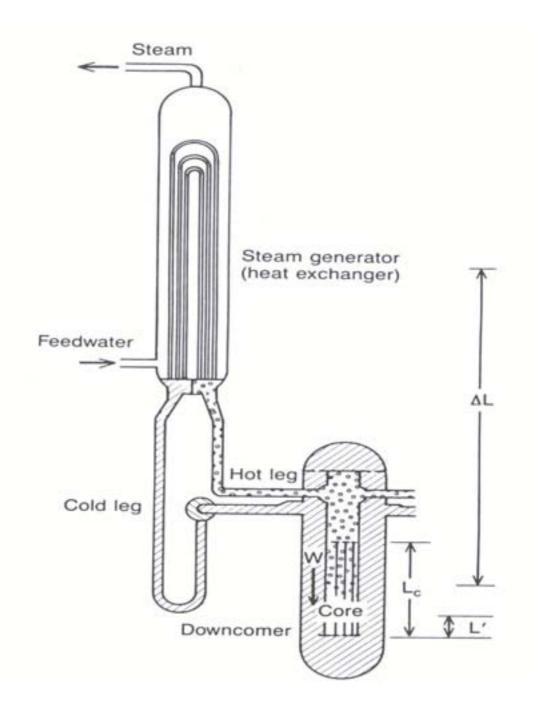
FIG.1. Schematic of a typical PWR system and elevations.
