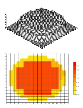
FIG. 8. Relative radial power distribution for the TMI-1 MSLB at SS, code run 10b (Relap5/Parcs code).
