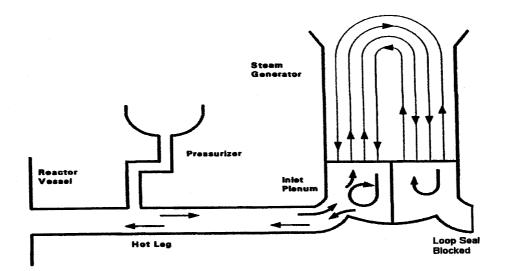
FIG. 9. Overview of natural circulation flow pattern in a hot leg of a PWR during severe accident conditions.
