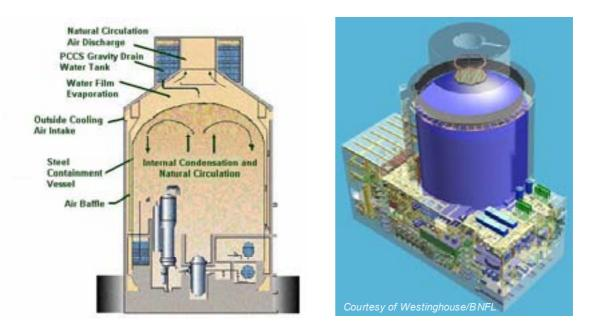
FIG. 3. AP1000 containment and passive containment cooling system (PCCS).
