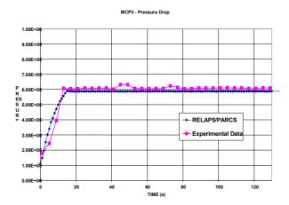
FIG. 38. Pressure drop in the MCP#3 zone.
