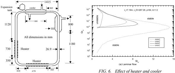
FIG. 5. Schematic of experimental loop.
