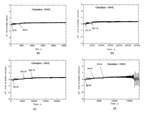
FIG. 14. Instability threshold for power raising from stable steady state.
