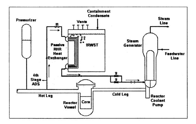
FIG. 2. The AP600/1000 Passive residual heat removal system (PRHR) using a heat exchanger connected to the primary system and immersed in the IRWST.
