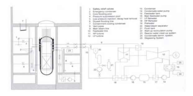
FIG. 10. Schematics of the HPLWR primary circuit, safety systems and containment concept.
