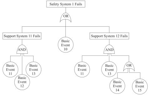
FIG. 5.3. An example of a fault tree.
