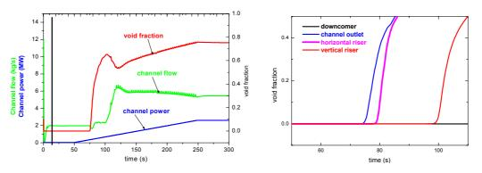
FIG.21. Simulation of power raising procedure from hot shutdown condition.
