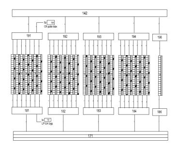
FIG. 32. RELAP5 core nodalization.
