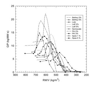
FIG. 2. Natural circulation system behavior measured in ten experiments performed in six PWR simulators.
