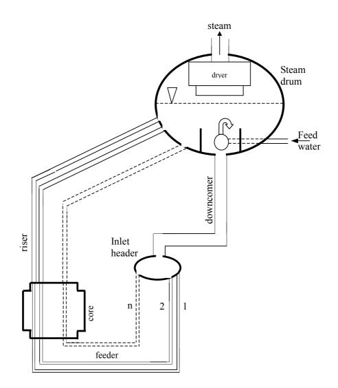
FIG. A-1.1: Schematic of AHWR system.
