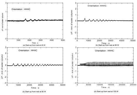
FIG. 13. Instability threshold for start-up from rest.
