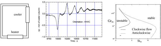
(a) An asymmetric NCL (b) Flow initiation in anticlockwise direction (c) Stability map
