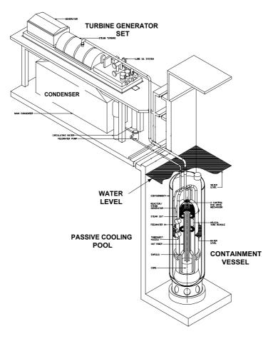
FIG. A.1. Schematic of the MASLWR exterior cooling pool and turbine-generator set.
