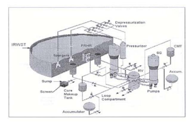
FIG. 1. Schematic of the passive safety systems used for the AP600/AP1000 designs.
