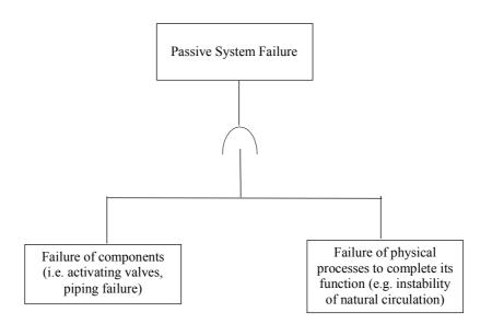
FIG. 5.4. Frame of a passive system fault tree.
