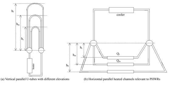
FIG. 10. Parallel channel systems.
