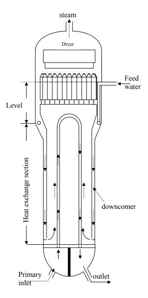
FIG. 22. NC based nuclear steam generator.
