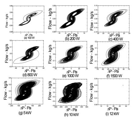
FIG. 25. Predicted limit cycles for different powers.
