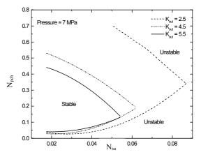
FIG.11. Effect of outlet orificing on DWI.
