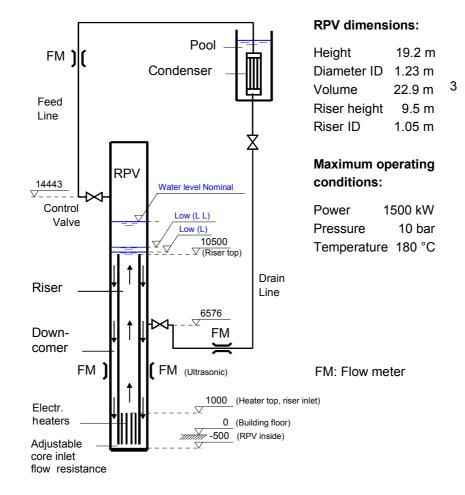
FIG. 11. PANDA experimental facility, natural-circulation loop and condensation/cooling loop (NACUSP) configuration.
