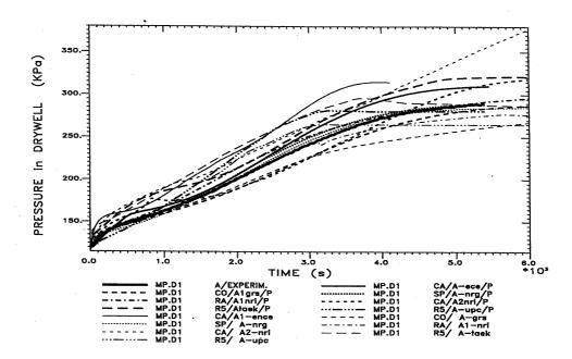
FIG. 6. Comparison of drywell pressure calculations (blind and open phases) with experimental data for Phase A of ISP-42.
