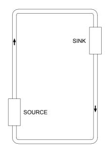
FIG. 1. A rectangular closed natural circulation loop.
