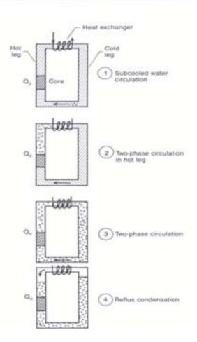
FIG. 6. Different modes of natural circulation cooling in a PWR..
