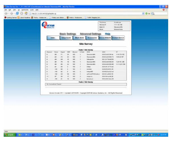
All Qnodes within a mesh, are visible from any Qnode within the mesh:
