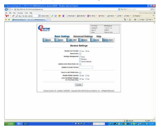
The technician simply loads the name of the desired update into the Update field, hits the Update button, and the node automatically contact the Qorvus server, and after validation, the new upload is installed automatically in the background. Often, the can take place with no reboot or interruption in user traffic.
