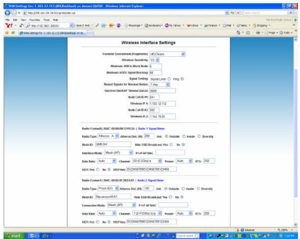
All important parameters for Atheros and Prism based radios such as the Wistron CM9, Ubiquiti SR-5 and SR-9, and Senao mp2511 are supported including wireless IP, standard ISM and UNI-1 channels from 900 Mhz to 5.8 Ghz, ESSID, link distance, encryption, fragmentation, transmit power, and receive sensitivity.
