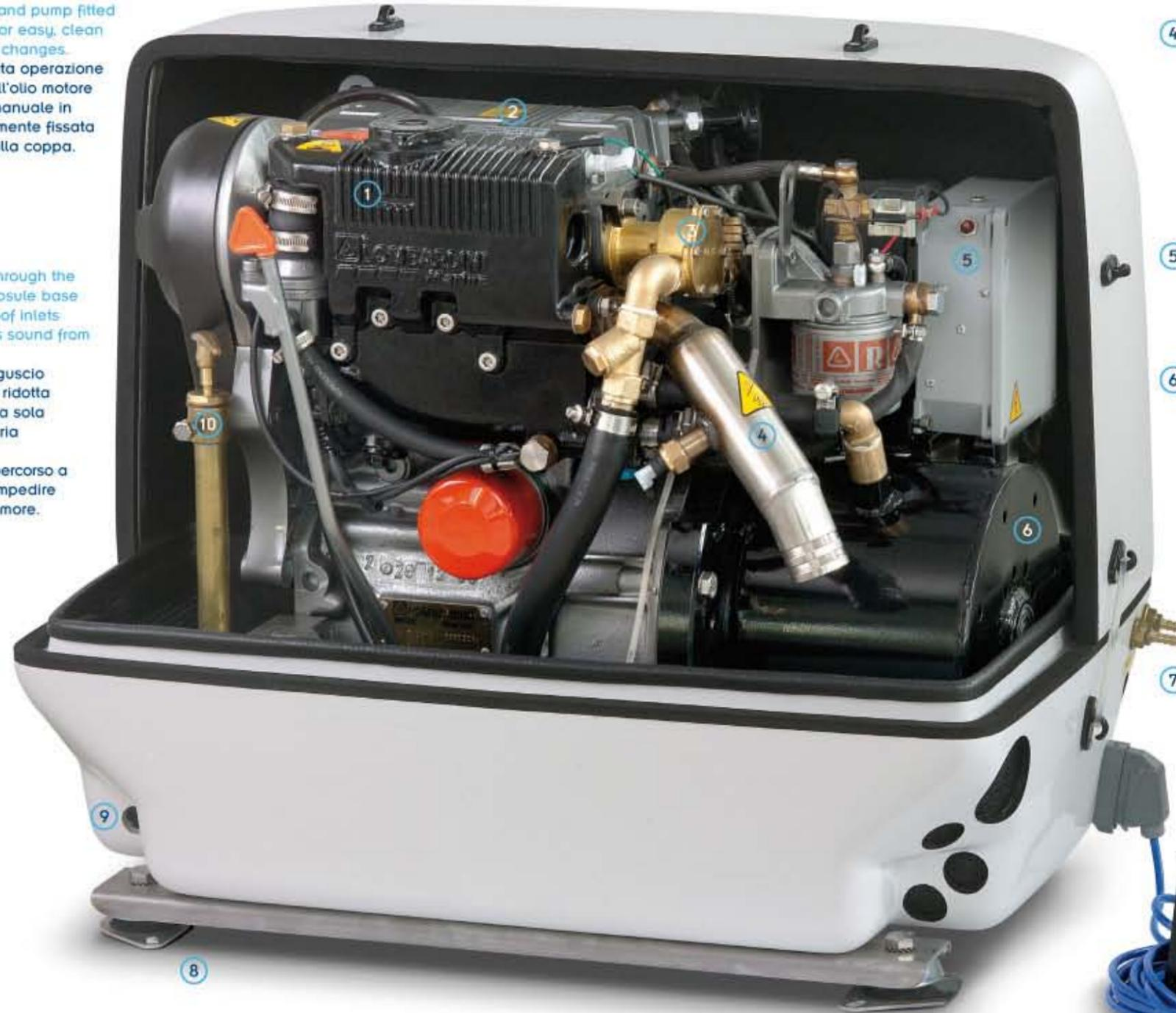
4 Exhaust and sprayed water manifold completely in stainless steel with high surface area cooling jacket. The cooled wet exhaust system ensures that no heat or vibration is transferred through the 45 mm. rubber hose.
