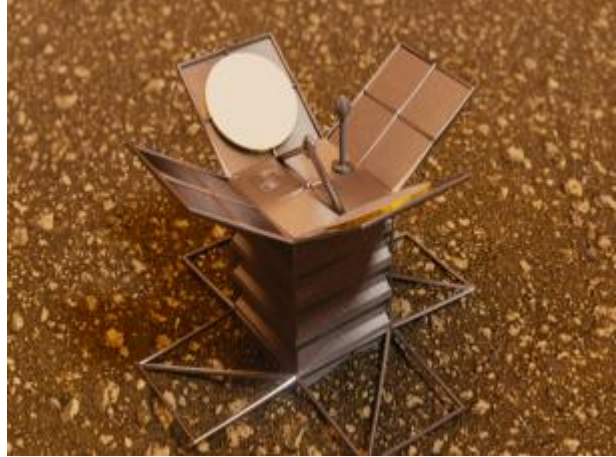
Figure 7.2-1. Concept for a small long-lived station that would operate on the surface of Venus for up to at least 60 days to make measurements of pressure, temperature, wind, and atmosphere composition.
