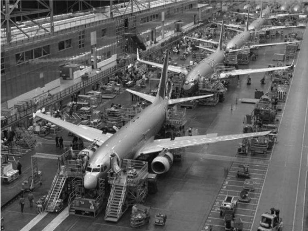
Figure 8. Boeing produces one $200 million plane per day in massive production lines that could be a model for mass production of liquid fluoride thorium reactors. Centralized mass production offers the advantages of specialization among workers, product standardization, and optimization of quality control, as inspections can be conducted by highly trained workers using installed, specialized equipment.
