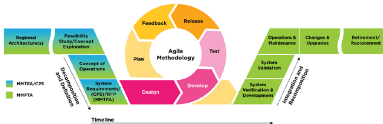
Figure 8-4: MMTPA/CPS Hybrid Systems Engineering/Agile Development Methodology
