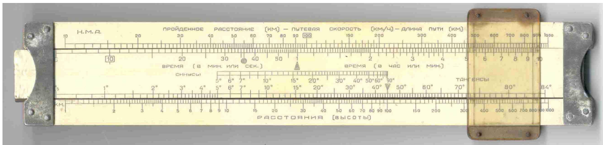
Figure 50 Soviet NL-7 flight computer {RvR}
