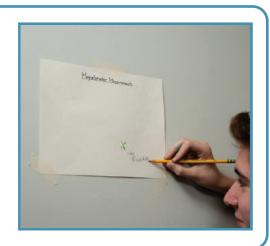
Record the postion of the bright dot on the white paper two to three times throughout the day for 3 days. The movement of the laser beam indicates a change in solar activity! A large increase in solar activity will influence Earth's magnetic field and the position of the laser dot.
