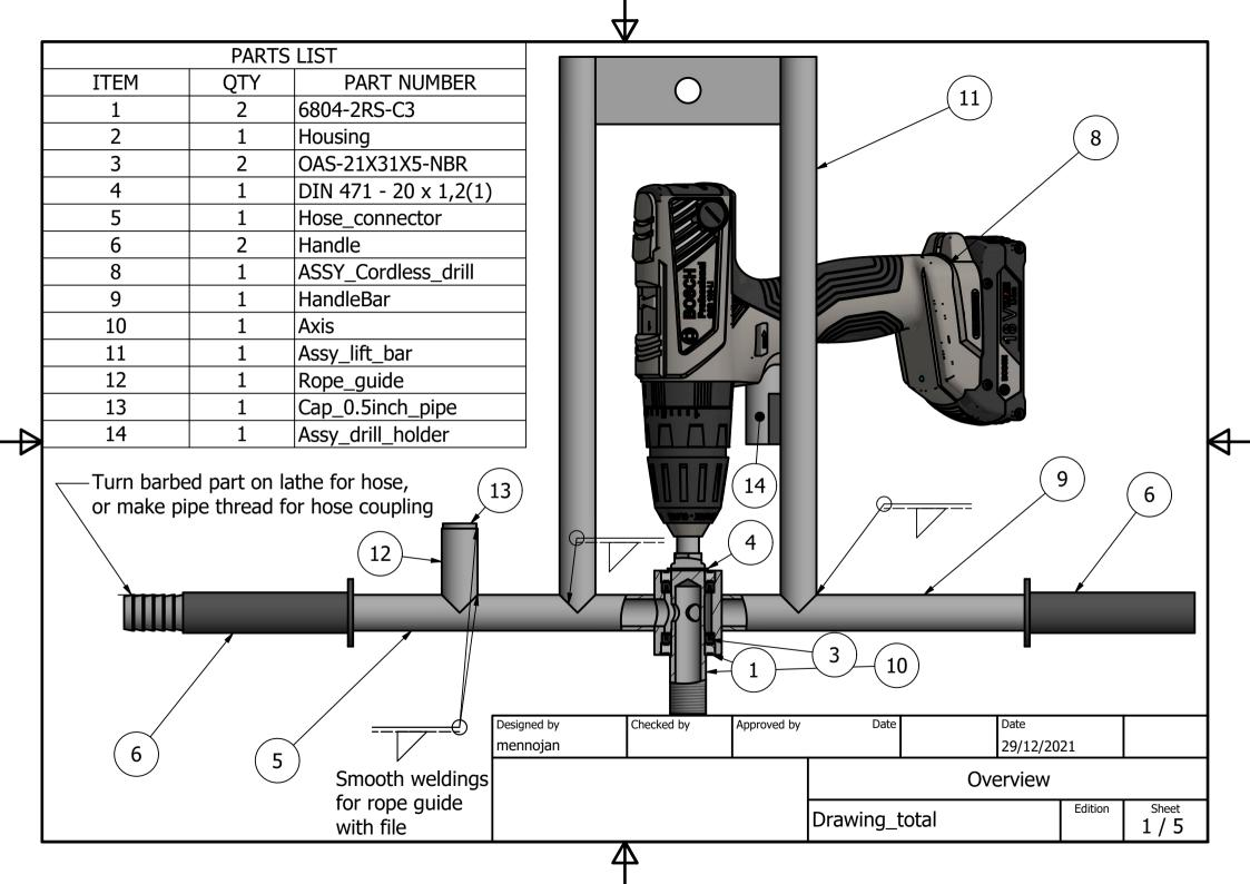
Drill actuation can be done with brake lever (bicycle), or rotating handle (accelerator motorcycle). Details are not specified, as it depends highly on used drill and type of handle.
