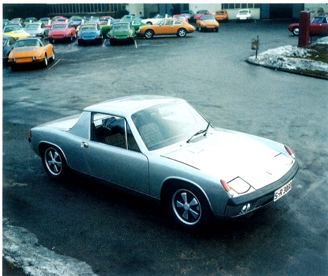
ABOVE, LEFT: The subtle silver 914-8 built for Ferry Porsche looked far more like the production 914 than Piëch's car, but was a true, all-steel coupe with a sunroof. Note also its separate fuel-filler door. ABOVE, RIGHT: Klie's unusual 914-4 is currently being restored in Germany. Stay tuned...
