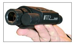
The PT2 thermal monocular is an uncooled micro-bolometer operating in the long-wave infrared (LWIR) spectrum, with three variations available. In service with the GRU.
