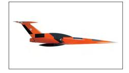
The Blik-M is a jet-propelled recoverable aerial target developed by Aerotechnica Ltd. It was developed to be operated as a high-speed target for multiple gun- and air-defence missiles. The AV is fitted with an aerial target imitator that can simulate airborne threats with a radar cross section between 0.1 m2 and 100 m2.
