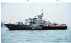
The MR-352 (Positiv-E or Pozitiv-E – suffix 'E' for export) is an S-band (NATO E-/F-band) (2–4 GHz) two-dimensional target-acquisition and fire-control radar meant for installation on board surface ships. NATO reporting name 'Cross Dome'. Used by the Russian Navy
