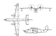
The Beriev Be-12 (M-12) Chaika (Seagull) is an amphibious aircraft first developed in the Soviet Union in the 1950s. The aircraft is powered by two 3,862 kW (5,180 ehp) Ivchenko AI-20D turboprop engines, and is used in anti-submarine, maritime patrol, and search-andrescue operations. The aircraft features a cranked gull-wing, MAD boom, and can accommodate a crew of five.
