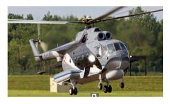
The Mil Mi-14 is a development of the Mi-8 helicopter generally for maritime operations. Mi-14 retains a number of features in common with the Mi-8 but also adds additional antisubmarine (ASW) capabilities. The Mi-14 has a new power plant, with a flotation bag carried in a sponson, with floats under the tailboom. The first prototype flew in 1969 and a number remain in service with countries worldwide.
