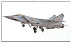
The MiG-31 is a supersonic multirole aircraft developed and manufactured by MiG (Inzhenirnyi Tsentr 'OKB Imeni A I Mikoyana'). The aircraft was developed in late 1960s as a long-range, extended-endurance PVO interceptor to replace the Tu-128 and MiG-25 and to counter the threat of the United States Air Force (USAF) B-52 bombers carrying ALCMs. Equipped with two low-bypass turbofan engines, the aircraft can carry out low-level supersonic flights, which MiG-25 lacked.
