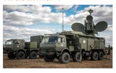
The Krasuha-4 is a broadband multifunctional jamming system designed to neutralise low earth orbit (LEO) spy satellites such as the US Lacrosse/Onyx series, satellites, ground-based radars, airborne surveillance radars, and radar-guided ordinance at ranges between 150–300 km. The complex functioning is based on creating powerful jamming at the fundamental radar frequencies and other radio-emitting sources.
