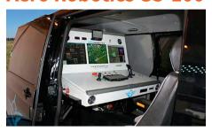
The GS-100 GCS is an ergonomic control station developed by Aero Robotics and integrated into a multi-purpose vehicle (MPV), from where it can be operated. The GCS controls up to two UAVs simultaneously, and can accommodate up to two crew members. It is developed by OOO Aero Robotics, Russia.
