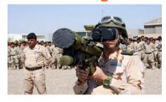
The 1PN97M Maugli-2M (Mowgli-2M) is a thermal imaging sight for the shoulder-launched 9K38 Igla (SA-18 'Grouse') and 9K338 Igla-S (SA-24 'Grinch') MANPADS, as well as the Dzhigit twin-launcher and Strelets double-quad AFV-mounted system, which use the same missile. In service with the Russian Army.
