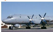
The Il-38 is a maritime patrol aircraft which was manufactured by Ilyushin in Russia. The aircraft is based on the four turboprop engine powered Il-18 airframe. Development of Il-38 was initiated in 1960 and the first aircraft was delivered in 1967. Versions of the platform continue to be in operation with the Russian and Indian Naval Forces.
