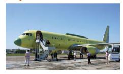
The twin engine PS-90A powered Tu-214 platform has been modified by Russia to serve its strategic command post and communication relay duties. Note this platform is also covered under EW.
