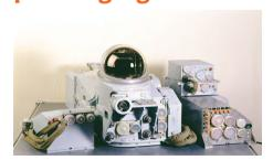
OEPS-29 and OPES-27 are infrared search-and-track (IRST) systems developed for early models of the MiG-29 'Fulcrum' and the SU-27 'Flanker' fighters, respectively. In service with both Russia and Ukraine.
