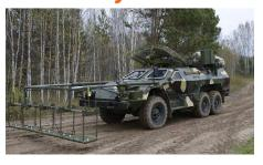
The BPM-97 Vystrel is a wheeled AFV based on a Kamaz chassis, designed for use with the Russian border guards. The vehicle was developed in the late 1990s and is now known to be in service with the counter-terror units that accompany Russia's strategic missile forces as well as elements of the Russian Special Forces.
