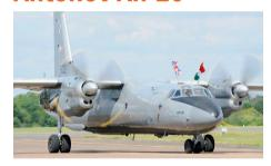
The An-26 is a twin-turboprop pressurised short-haul transport, manufactured by Antonov, in Ukraine. The aircraft is based on the earlier An-24RT and has an extended fuselage tail section with large cargo door and ramp. was first exhibited in 1969 and was superseded by the An-32 after 1986.
