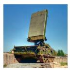
The 1L220U, 1L220UK, and 1L220U-KC are S-band (NATO E-/F-band) (2–4 GHz) mobile battlefield 3D phased-array fire-control radars designed to establish the co-ordinates of hostile artillery, mortars, multiple launch rocket systems, and tactical missile batteries, provide targeting data for counter-fire operations and monitor friendly fall of shot.
