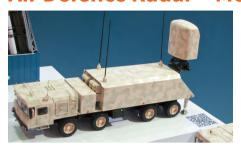
The Monolit-B is a coastal surveillance radar for surface and air reconnaissance to provide target designation to land-based, anti-ship missile systems such as the K-300P 3M55 Bastion-P mobile coastal defence missile system, the Bal-E 3K60 Kh-35E Uran, and the Club-M missile systems.
