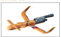
The E17M series are recoverable aerial targets manufactured by ENICS. Three versions are publicised by the company: the E17MP, E17MV, and E17MT. The versions primarily differ in their powerplant and airframe size.
