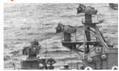
The 'Sprut''or 'Drakon' (NATO designation 'Eye Bowl') is an S-band (NATO F-band) (3–4 GHz) 3D tracking radar meant for installation on board medium and large surface ships. The radar is associated with the SS-N-14 ('Silex') long-range anti-submarine torpedo delivery system. In service with the Russian Navy.
