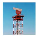
The RSM 970 S is an L-band (NATO D-band) (1–2 GHz) mode S monopulse secondary surveillance radar (MSSR) meant for air traffic control that can be operated stand-alone or co-mounted with a primary surveillance radar.
