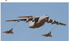
The Il-78 is a tanker/transport aircraft based on the four-engine Il-76MD airframe and is manufactured by Ilyushin in Russia. Development began during the 1970s with entry into service in 1987. The Il-78 is used for aerial refueling and freight missions. The Il-78 is in service with a number of countries worldwide, with new-build versions ordered.
