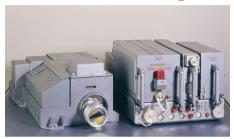
The Prichal is a laser rangefinder/designator. It is a subsystem of the I-25I Shkval targeting system (see separate enrtry). In service with both Russia and Ukraine.
