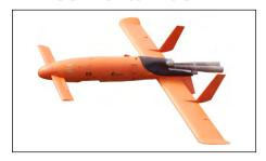
The ENICS Berta E08 (sometime referred to as Berta E08M) is an aerial target, manufactured by JSC ENICS of Russian Federation. It is designed to simulate remote piloted vehicles (RPVs), aerial-guided bombs and cruise missiles for testing weapon systems and training of the personnel.
