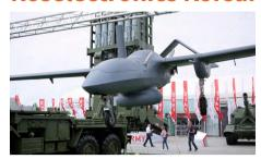
The Korsar is a medium-sized fixed-wing unmanned aerial vehicle (UAV) designed by the Lutch R&D company of the Roselectronics holding (part of Rostec), Russia. The AV can perform ISR and strike missions in all-weather terrain.
