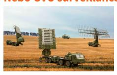
The 1L119 Nebo-SVU is a very high frequency (VHF) band (NATO A-/B-band) (30–300 MHz) long-range 3D volume mobile air surveillance radar meant for long-range detection of air-borne targets.
