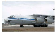
The Il-76 is a four-engine, strategic transport aircraft manufactured by Ilyushin in Russia. The current production Il-76MD-90A is an improved production version over the original Il-76, with Aviadvigtel PS-90A-76 turbofan engines, redesigned wings, strengthened landing gear and a glass cockpit. The Il-76MD-90A first flew in 2012 and was delivered in 2015. A tanker version, Il-78M-90A, is also produced based on the new production Il-76MD-90A airframe.
