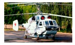
The Ka-35 also known as Ka-31SV/Ka-252CV was developed for ground-based radar reconnaissance. It is designed to detect ground based targets (both moving and static objects). The development of the Ka-31SV helicopter is being carried out by Kamov JSC of the Gorkovchanin R & D project, in the interests of the Russian Ground Forces as a further development of the Ka-31 naval shipborne helicopter.
