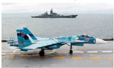
The Su-33 is a Russian all weather, carrier-based air superiority fighter designed by AVPK Sukhoi and manufactured by the Komsomolsk-on-Amur Aircraft Production Association. It is derived from the Su-27 and was initially known as the Su-27K. A two seat trainer variant was later developed, known as Su-33UB.
