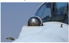
The Optiko-Lokatsionnaya-Stantsiya (Optical Locator Station: OLS)-UE/-UEM, developed for the latest variants of the MiG-29 (MiG-35), provides capability for search, detection, tracking, and ranging of airborne and ground targets. In service with Russia.
