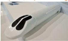
The Sapsan (Russian for peregrine) is a targeting pod originally designed to be fitted to the MiG-29 and Su-27/30 series of fighters. In service with Russia.
