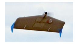
The ZALA 421-08 AV is a short-range reconnaissance and surveillance mini-unmanned aerial vehicle (UAV) manufactured by Zavod A-Level Aerosystems (ZALA) Aero Group (part of Kalashnikov Group since January 2015). The baseline version, ZALA 421-08, was revealed in 2007. The advanced version ZALA 421-08M mini-UAV was successfully tested at the MAKS-2013 air show at the training camps of the Russian MVD air detachments and at the joint Rosatom tactical and special exercises.
