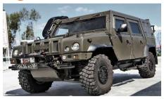
The Light Multirole Vehicle (LMV) is a 4×4 protected mobility platform designed to provide users with a general utility vehicle that can be used as a patrol vehicle or command-and-control platform among other things. It has been introduced into service with multiple users and developed into several different variants.
