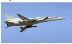
The Tu-22M is a supersonic strategic and maritime strike bomber developed and manufactured by Tupolev in Russia. The Tu-22M was developed to meet a Russian Air Force requirement for a variable geometry bomber from 1962 onwards and is based on the earlier Tu-22. The Tu-22M is designed to carry stand-off missiles, cruise missiles or free-fall munitions, depending upon the mission requirement and has been progressively upgraded through its service life.
