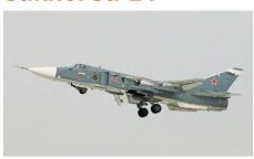
The Sukhoi Su-24 is a supersonic, all weather attack fighter featuring variable geometry wings, twin afterburning engines and a crew of two. Subsequent variants have been developed for reconnaissance and electronic warfare. It was designed in the 1960s and remains in service with Russia and several countries to which it was exported.
