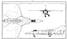
The MiG-27 is high-speed low-level ground attack aircraft developed and manufactured by MiG (Inzhenirnyi Tsentr 'OKB Imeni A I Mikoyana'). The aircraft structure is based on the same basic airframe of MiG-23 but with a revised nose. The aircraft was also licenced produce in India by Hindustan Aeronautics Limited. Versions of the MiG-27 are in service with the armed forces of Kazakhstan and Sri Lanka.
