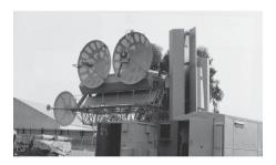
The RSN-75 (NATO reporting name 'Fan Song') is a family of S-/C-band (NATO F-/G-band) (2–4 GHz and 4–8 GHz) target detection and missile guidance radars that have been developed for use with the S-75 (NATO reporting name SA-2 'Guideline') surface-to-air missile (SAM) system. In service with both Russia and Ukraine.
