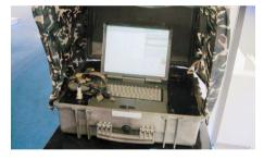
The automated MANPAD C2 system provides command and control (C2) for up to nine firing units of shoulder-launched AD weapons. In service with the Russian Army.
