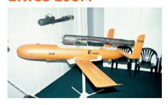
The ENICS E95M is a pulse jet-powered, subsonic aerial target designed to test and evaluate anti-aircraft weapons as well as train aerial gunnery crews. It was developed and manufactured for the Russian Armed Forces by ENICS in Russia. The E95M simulates a range of potential targets and mimics the maneuvering characteristics of simulated threats such as aerial bombs, cruise missiles, fixed-wing and rotary-wing aircraft.
