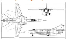
The MiG-23 is a multirole fighter aircraft developed and manufactured by MiG (Inzhenirnyi Tsentr 'OKB Imeni A I Mikoyana'). The development programme began in 1964 with an intention to replace MiG-21s. The MiG-23, with MiG-27, superseded MiG-21 as primary equipment in Soviet tactical air forces and APVO home defence interceptor force. The shoulder mounted sweep-wing feature augments the operational capability of the aircraft during combat missions.
