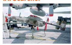
The Searcher is a family of long-endurance, multi-role unmanned aerial vehicles (UAVs) designed and manufactured by Israel Aerospace Industries (IAI). The first production Searcher AV had been rolled-out during November 1991. It is used for surveillance, reconnaissance, target acquisition, artillery adjustment, and damage assessment.
