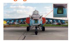
The Klyon laser rangefinding and designator provides measurement of range and can be used in different fighter aircraft. In service with both Russia and Ukraine.
