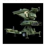
SNR-125 forms part of the Almaz S-125 Pechora (NATO reporting name SA-3 'Goa') surface-to-air missile (SAM) system and is designed to guide missiles against low-flying targets operating in heavy clutter conditions. In use by both Russia and Ukraine.
