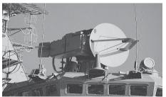
The MR-114 Lev, MR-145 Drakon, and MR-184 are X-band (NATO I-band) (8–10 GHz) and Ka-band (NATO K-band) (27–40 GHz) 3D fire-control radars meant for installation on board surface ships. NATO reporting names 'Kite Screech' (MR-114), 'Kite Screech A' (MR-145), and 'Kite Screech B' (MR-184). In service with both the Russian and Ukrainian navies.
