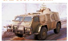
The GAZ-3937 series of 4 × 4 light armoured vehicles (LAVs), also referred to as Vodnik, was developed by the Arzamas Machinery Plant as the basic member of a complete family of LAVs, which could be used for a wide range of paramilitary and military roles.
