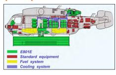
The E-801 Oko is an ultra-high frequency (UHF) band (NATO C-band) (0.3–1 GHz) 3D airborne early warning (AEW) and surface surveillance radar meant for installation on board the Kamov Ka-31 helicopter (NATO reporting name Helix-B). In service with Russia.
