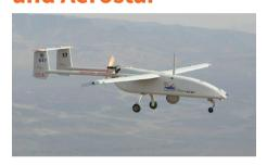
The Aerostar TUAV series (Aerolight, Aerosky, and Aerostar) are close range unmanned aerial vehicle (UAV) designed and manufactured by Aeronautics Defence Systems Ltd. The Aerolight and Aerosky are small UAVs, with the Aerostar being a tactical UAV. The Aerostar family was introduced in 2000 and is in service with a number of civil and military operators. The primary mission role of the Aerostar family is reconnaissance, surveillance and over-the-horizon patrols.
