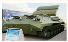
The 1L121E (suffix 'E' for export) is an ultra-high-frequency (UHF) band (NATO B-/C-band) 300 MHz-1 GHz mobile 3D radar meant for detection of air targets such as aircraft, drones, or precision-guided munitions.
