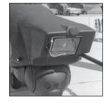
The I-25I Shkval sighting system is designed to detect, track, and identify fixed and moving ground targets and slow airborne targets. Out of production but assessed to still be in use with Russian Air Force.
