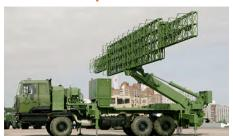
The Vostok-D/E is a VHF-band (NATO A-band) (175 MHz centre frequency) 2D ground mobile air defence early warning radar. The system is designed to replace the Sovietera P-18 'Spoon Rest D' radar in Belarusian service.
