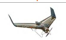
The AEROKON INSPECTOR 2020 is a recoverable aerial target developed by AEROKON in Russa for Man-Portable Air Defence Systems (MANPADS) training. The INSPECTOR 2020 completed flight trials in 2012 and entered testing during 2014.
