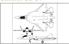
The Su-57 is a Russian multirole, single-seat stealth fighter aircraft. It is a fifth-generation aircraft made primarily of titanium alloy and equipped with twin-engines having independently-moving thrust vectoring nozzles. Development began as the PAK-FA in 1998 with first flight occurring in 2010 and low-rate initial production (LRIP) in 2019.
