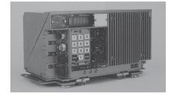
R-173M is a VHF tank radio providing transmission and reception of digital information in pulse mode. In service with both Russian and Ukrainian Armies.
