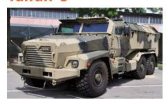
The Taifun-U is a family of MRAP vehicles developed by Ural Automotive to provide a wheeled MRAP capability for the Russian Armed Forces and export customers. The vehicles are at various stages of deployment and development.
