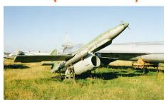
The Lavochkin La-17 is a subsonic aerial target, manufactured by PO Strela in Russia. It is a jet-powered target of all-metal construction and was developed as the first non-towed target in the Soviet Union. The target was initially developed to be ram-jet powered. Five distinct versions were produced.
