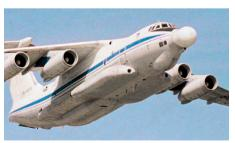
The A-60 is an airborne laser technology demonstrator platform developed by Beriev. It is based on the Il-76 transport aircraft. The A-60 is used for the airborne combat laser programme and houses a laser system in its cargo section. The initial platform A-60(1A) which first flew in 1981 was built as a reconnaissance balloon interceptor. Subsequent platform was known to have taken an anti-satellite role. The A-60 platform is still in the development stage and none are known to be operational.
