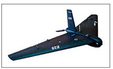
The dynamic simulation aerial target DSAS E25 is manufactured by ENICS. The DSAS E25 aerial target was developed to imitate F-16 and Tornado fighter aircraft silhouettes, angle, trajectory and speed on a scale 1:14 - 1:15. The E25 aerial target is deployed with the Igla missile system.
