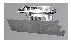
The Novella/Sea Dragon series is an X-band (NATO I-/J-band) (8–12 GHz) family of maritime surveillance radars meant for installation on board medium and large maritime rotary- and fixed-wing aircraft as well as aerostats.
