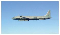
The Il-20 family is designed and manufactured by Ilyushin. The Il-20M and Il-20RT are based on the Il-18 transport platform which were built for the Russian Armed Forces. The first prototype was flown on 25 March 1968. The Il-20M is used for surveillance purposes, providing COMINT, SIGINT, and ELINT capabilities. The Il-20RT was used as a space/missile telemetry aircraft until its role was changed to transport and crew trainers.
