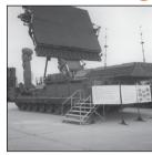
The 9S15MV Obzor-3 is an S-band (NATO F-band) (3–4 GHz) 3D target acquisition radar for the Antey S-300V surface-to-air missile (SAM) system. NATO reporting name Bill Board.
