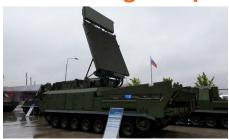
The 9S18M1 is an X-band (NATO I-/J-band) (8–12 GHz) 3D target acquisition radar associated with the Buk-M1 (NATO reporting name SA-11 'Gadfly') surface-to-air missile (SAM) system. NATO reporting name 'Snow Drift. In service with both Russian and Ukrainian air defence troops.
