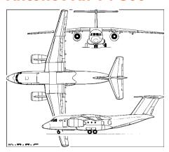
The An-74-300 is a twin-jet short take-off and landing (STOL) aircraft manufactured by Antonov in Ukraine. It is a modified An-74 fitted with underslung engines. The platform was introduced in 1998 and flew for first time in 2001. Versions were reported to be in service with Ukrainian and Libyan government.
