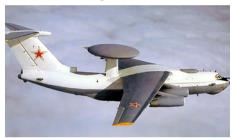
The A-50 is a family of airborne early warning and control system (AEW&CS) aircraft based on an Ilyushin Il-76 airframe, and manufactured by Beriev Aircraft Company. Its development began in 1969 with the development of the Shmel (Bumblebee) AWACS system, based on the Grib (Mushroom) radar. It features the rotating 'saucer' radome on twin pylons above the fuselage. Versions of the platform are currently in service with China, India, and Russia.
