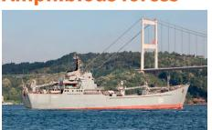
3 out 4 operational Alligator (Tapir) (Project 1171) class LSTM are part of the BSF. Lift capability include 300 troops; about 20 tanks and various trucks; 40 AFVs.
