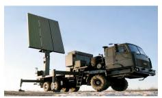
The Vostok 3S is an S-band (NATO E-/F-band) (2–4 GHz) 3D volume air-surveillance radar meant for ground-based air-defence systems and integrated C2 applications.
