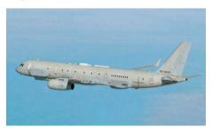
Russia mainly relies on multisensor variants based on its IL-20M and Tu-214R for its signal intelligence missions. Tu-214R is a multisensor platform uses the MRC-411 Fraktsiya multimission payload system onboard Tu-214R to intercept the signals of enemy Radars, communications systems and even cell phones to generate a real-time electronic map of the battlefield. It also includes imagery intelligence capabilities through TPC Linkos Electro-Optical (EO) imaging system.
