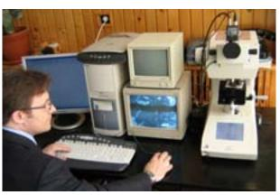
Vickers Microdurimeter controlled by computer
