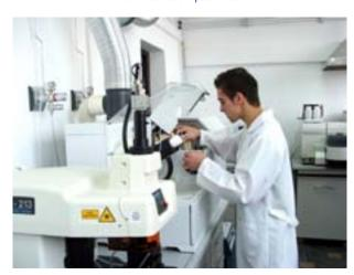
Atomic Emission Spectrometer with Mass Spectrometer and Laser Ablation
