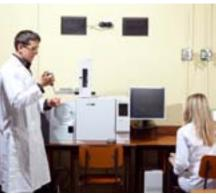
Gas Chromatograph with mass spectroscope
