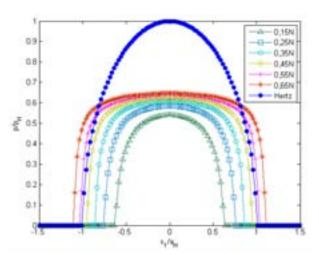
Pressure Distribution in Elastic-Plastic Spherical Contact
