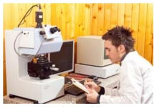
Martens Microdurimeter controlled by computer
