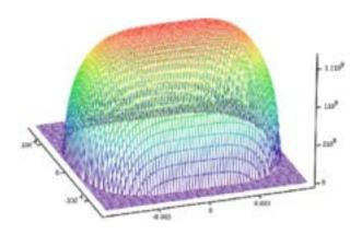
Improved pressure distribution in tapered roller contact
