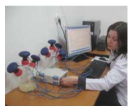
Fermentation Process monitoring with CO<sub>2</sub>-Ethanol-O<sub>2</sub> sensors
