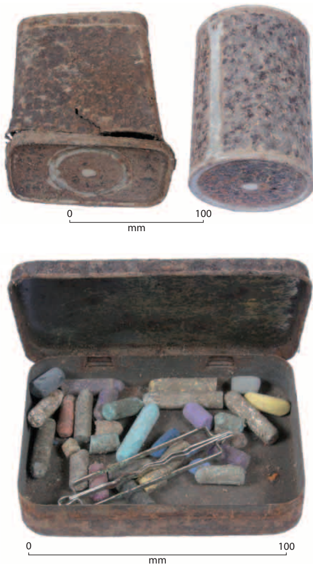
47 (top). Tin cans: left, 'hole-in-cap' rectangular tapered preserved meat can; right, cylindrical 'hole-in-top' food can (note the soldered seams on both cans).
