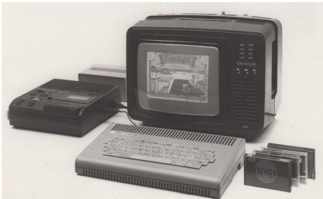
Figure 3.5. Santaka set including the main unit, TV, tape recorder, power supply and some software tapes (Saulius Matelionis's private collection)
