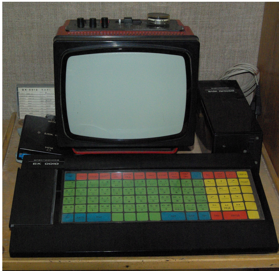
Figure 3.4. BK-0010 with display, power supply and software tapes (photo taken by the author)
