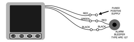
Figure 1 - Wiring Installation
