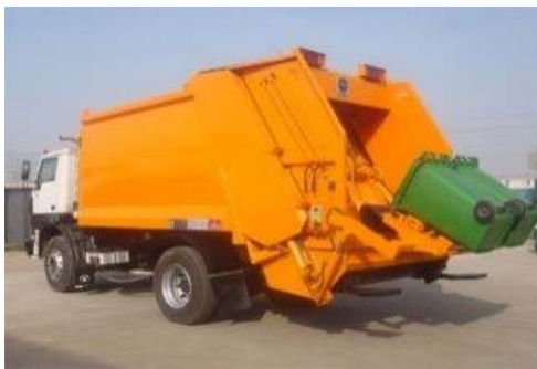
Plate 2.3: Utility Vehicles Rear Loaders (REL) Garbage Compactor Trucks
