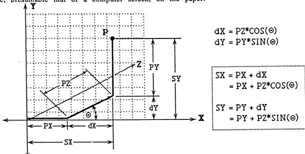
One can see that the transformation is achieved by a displacement of the x and y coordinates. If  $\Theta$  is the angle that the z axis makes with x axis (in two space,) and dx and dy are the x and y displacements, then it is clear that dx =PZ\*cos( $\Theta$ ), and dy = PZ\*sin( $\Theta$ ). Thus, the transformation of a point P from three space into the two space of the screen is simply:
