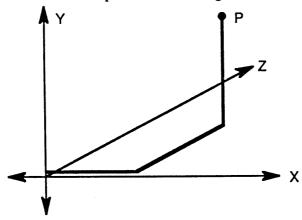
As you can see, this representation of a three dimensional space is completely embedded in the two dimensional space of the paper. The effect of three dimensions is achieved by placing the z axis at an angle between the x and y axes. The transformation follows directly if we imagine placing a two dimensional coordinate space, presumable that of a computer screen, on the paper:
