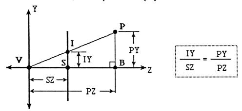
Using similar triangles, it is clear that IY=SZ\*PY/PZ. This same method is used to solve for IX, by looking down on the model from the top. Then, IX=SZ\*PX/PZ. Note that SZ is the distance of the screen from the x-y plane which was chosen arbitrarily. Changing the distance of the screen from the x-y plane alters the severity of the perspective. If the screen is close to the x-y plane, the perspective will be more dramatic than if it is farther away.
