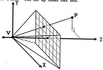
Transforming the point from three space onto the two space of the screen is really just a matter of drawing a line segment from the viewpoint to the point which is to be transformed and determining where this line segment intersects the screen. One way of doing this would be to determine parametric equations for the line segment
