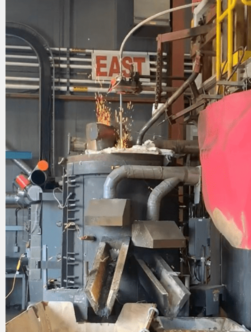
Converting NiCuCo alloy into NiCuCo matte (intermediate) at the same XPS facility.
