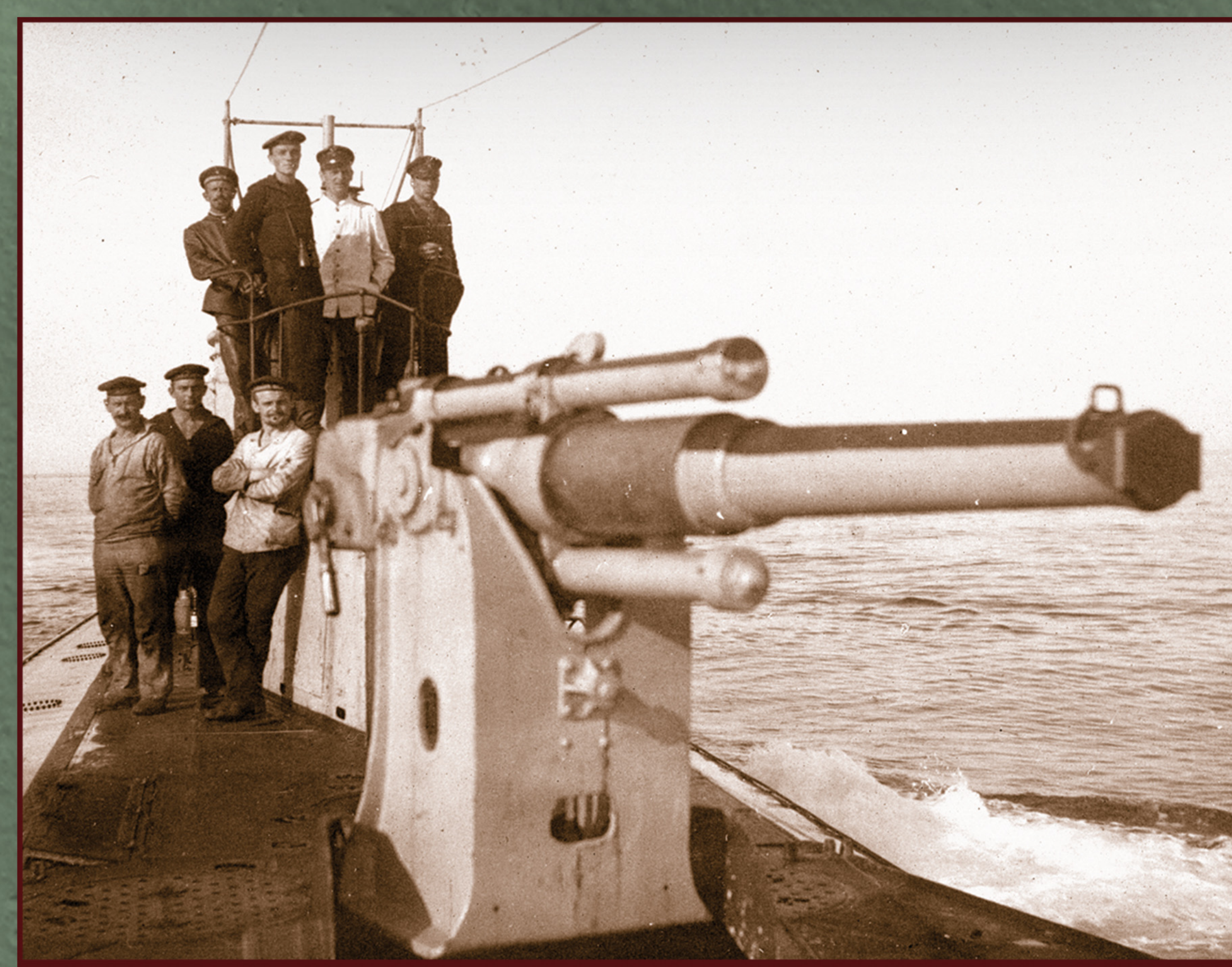
A U-boat's gun team poses with their weapon, a 105mm breechloading rifle. To conserve vital torpedoes, which were the submarine's main weapon, U-boat skippers used the deck gun whenever they deemed it safe to surface.
