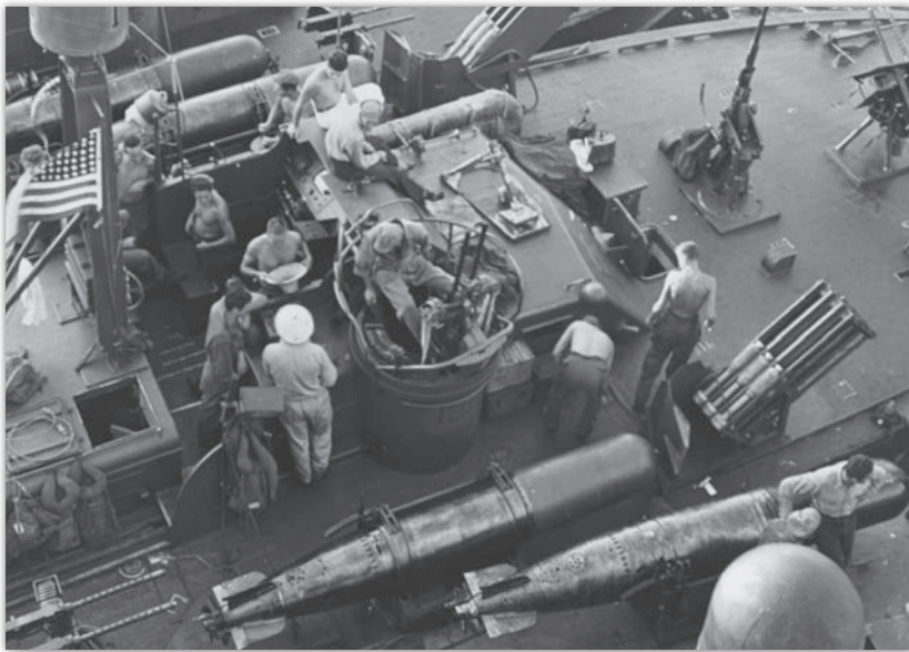
PT-131 (foreground) and other motor torpedo boats prepare for the Battle of Surigao Strait on 24 October 1944. Note the Mark XIII torpedoes, rockets, mortar (atop PT-131's forward deckhouse), 20mm machine cannon and 50-caliber machine guns carried by these PT boats. (NARA, NHHC 80-G-345819).
