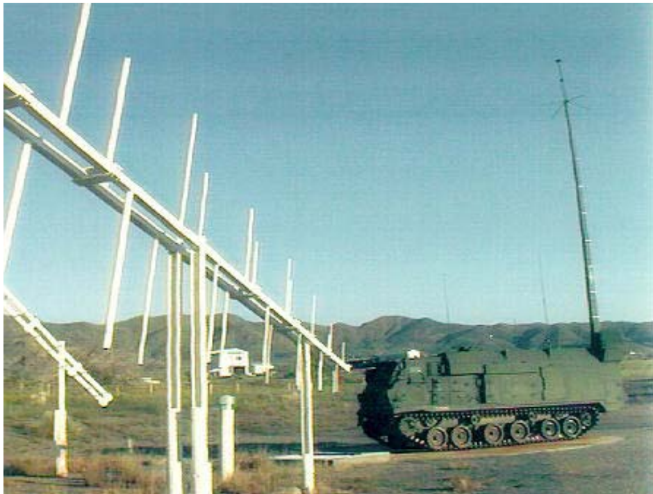
Figure C-2. (U) Generic Long Antenna VEMP Test Setup.
