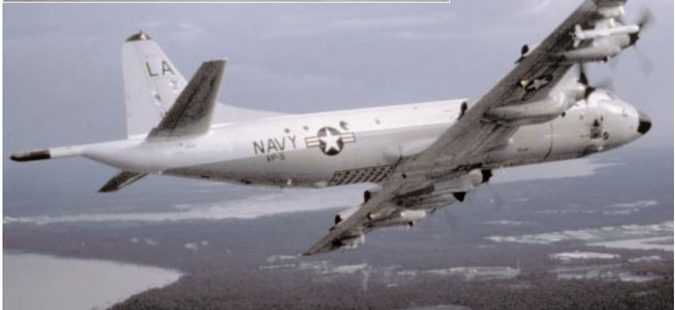
A squadron P-3 Orion in flight with a Harpoon missile under the wing.
