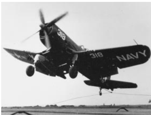
A squadron F4U-4 Corsair catching the wire aboard Philippine Sea (CV 47) during their 1951-1952 combat deployment to Korea.
