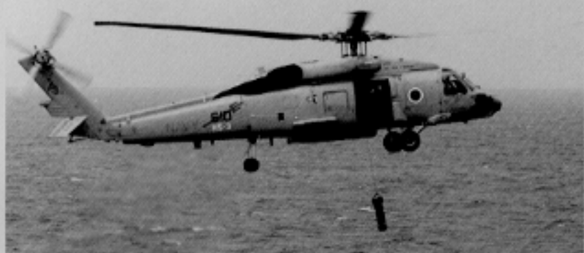
An SH-60 Seahawk from HS-3 dips its sonar buoy during flight operations in the Red Sea.
