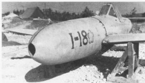
As they took over former Japanese installations, American soldiers discovered several examples of unused Ohka suicide rocket planes; this one was found on Okinawa. Crude in construction, the Ohka was an unusual weapon that "enjoyed" some success. The forward fuselage was reserved for the large warhead. Note the primitive ring-and-bead gunsight just forward of the windscreens.
