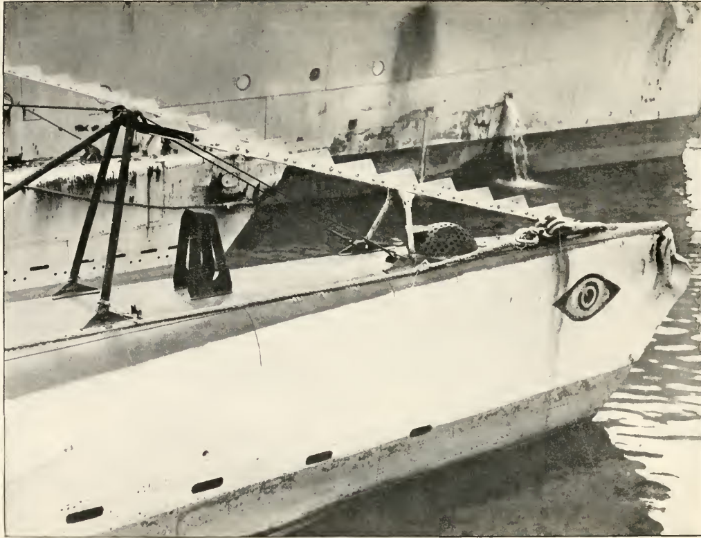
GERMAN U-BOAT SHOWING SAW-TEETH ON THE BOW USED FOR CUTTING NETS.
