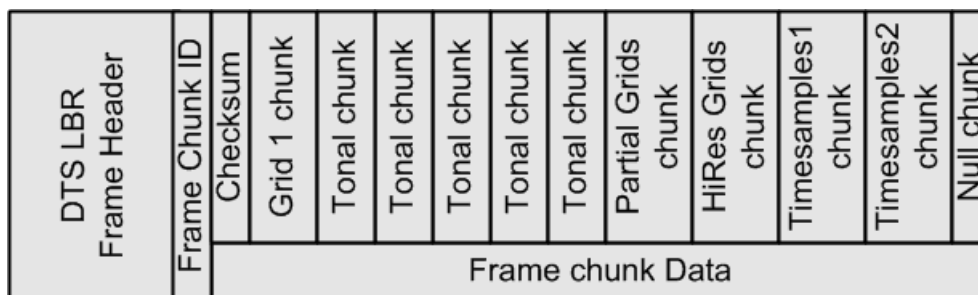
Figure 9-1: Generalized LBR Frame
