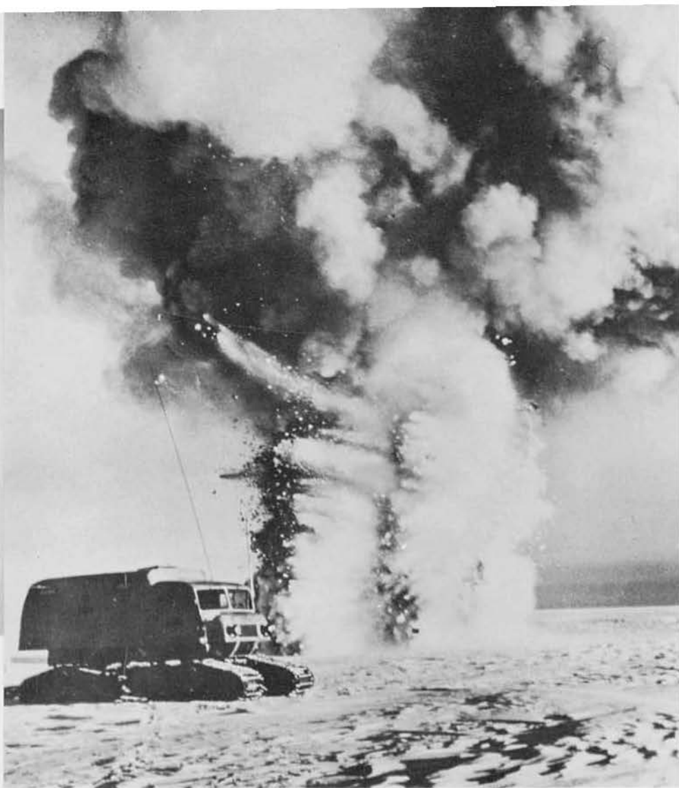
SEISMIC explosion (above) sends shock waves downward to bedrock below ice; echoing back to surface they are picked up by electronic receiver (top right) which amplifies and records shock data. Time interval between shock and sound's return indicates thickness of ice. Glaci-
