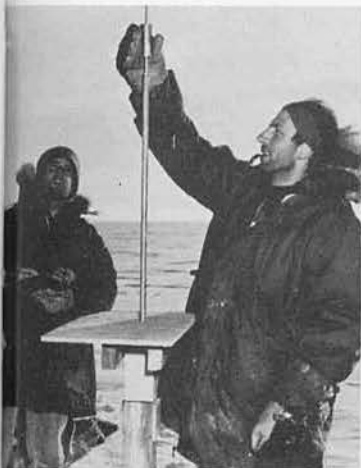
← IGY scientists Walter Boyd and Peter Shoeck test the density of snow with ramsonde equipment (left) as Al Crary drills for core samples of the vast ice shelf. Crevassed areas were source of data on stratigraphy.
