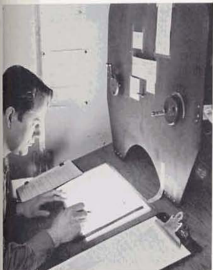
FILM RECORDS from ionospheric recorder are scaled, evaluated. Far right, portion of ionosphere trace as recorded on film by photoelectric equipment.
