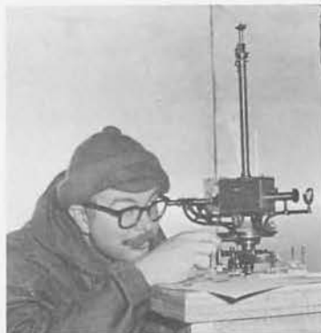
GEOPHYSICISTS doublecheck: Carl Wyman eyes ionospheric film, Ronald Viets calibrates geomagnetic piers.
