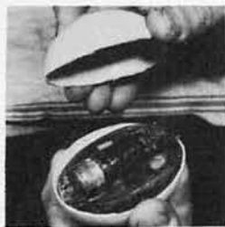
TEMPERATURE telemeter placed in penguin eggshell tells scientists incubating heat of nesting penguin. Carl Eklund (above, right) and assistant Fred Charlton of Wilkes prepare "bugged" egg, slip it under co-operative bird, orient antenna, read panels of telemeter (shown above).
