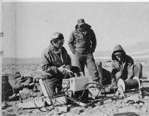
SEISMOLOGISTS and glaciologists pooled talents to study earth's inner core. Preparing seismic blast (left); determining density of ice (center) by weighing ice core mined from snow pit.
