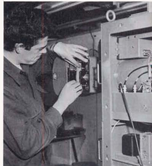
IONOSPHERIC research tools are mainly a sounder, sending radio signal to ionosphere, and a recorder, making film and tape records.
