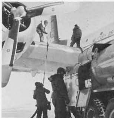
PLANES were gassed up on runway (right) by big tank trucks which got their supply of avgas from three-mile fuel line extending from storage tanks to flight line.
