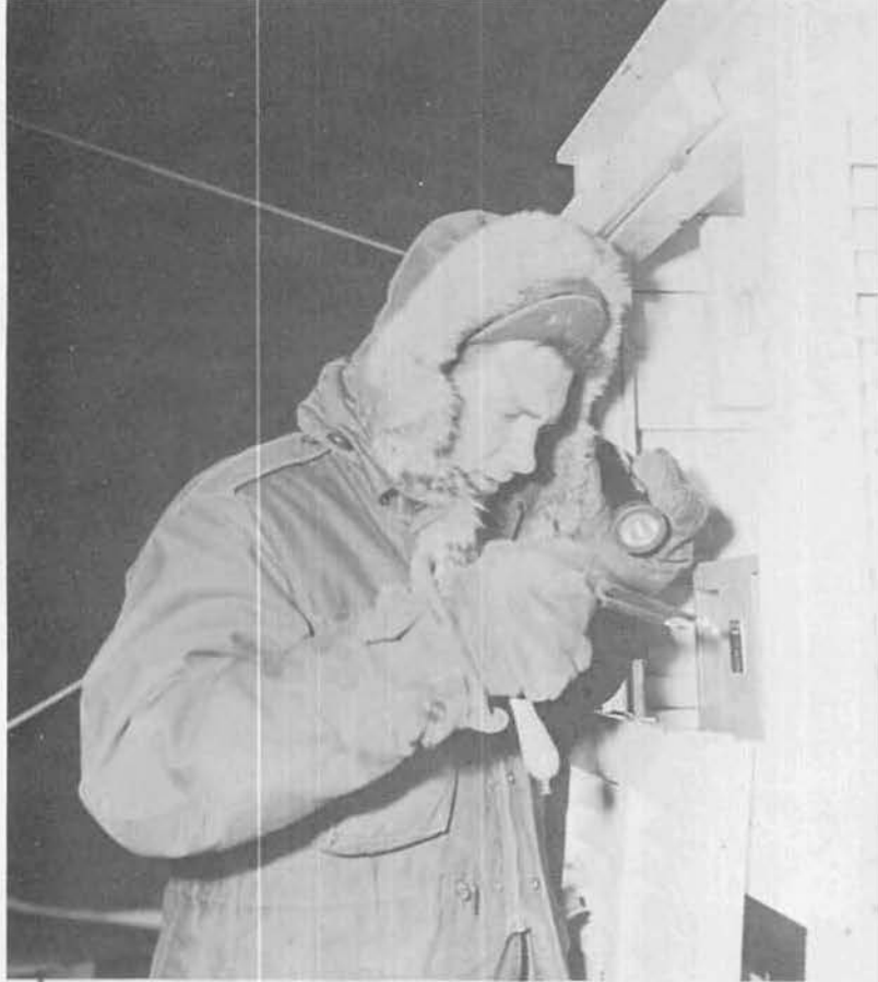
SLING psychrometer reading, determining humidity, is taken from inside instrument shelter atop aero shack by Navy aerologist Lilienthal during hours of dark at Wilkes.
