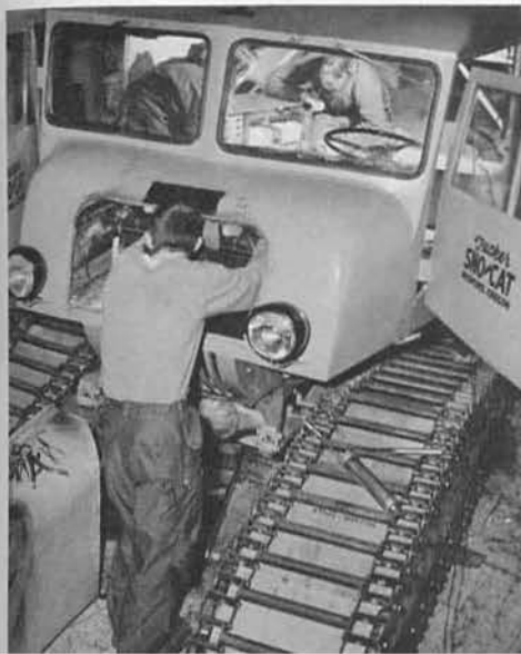
OVERLAND travel was by aluminum-cabbed Tucker Sno-Cat (above) driven by 180-hp engine. Otters provided air shuttle service here being mapped out by CO and VX-6
