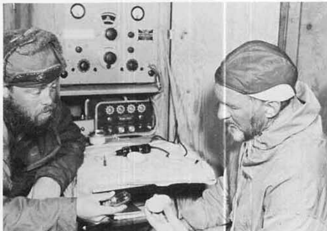
TEMPERATURE telemeter placed in penguin eggshell tells scientists incubating heat of nesting penguin. Carl Eklund (above, right) and assistant Fred Charlton of Wilkes prepare "bugged" egg, slip it under co-operative bird, orient antenna, read panels of telemeter (shown above).
