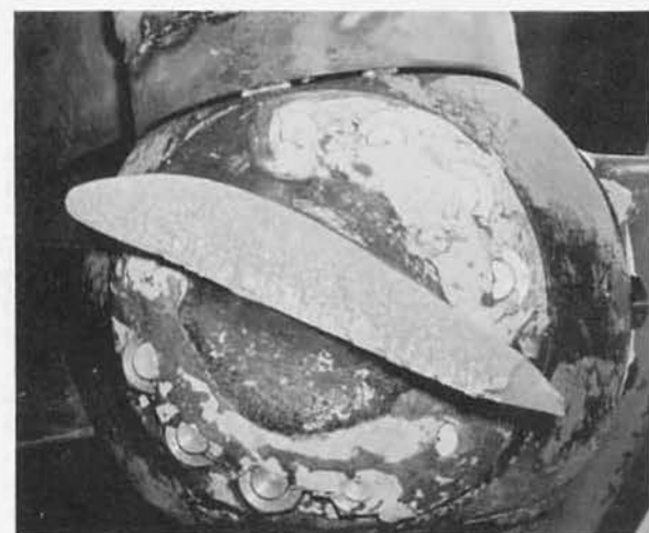
STUB OF BROKEN PROPELLER BLADE.
