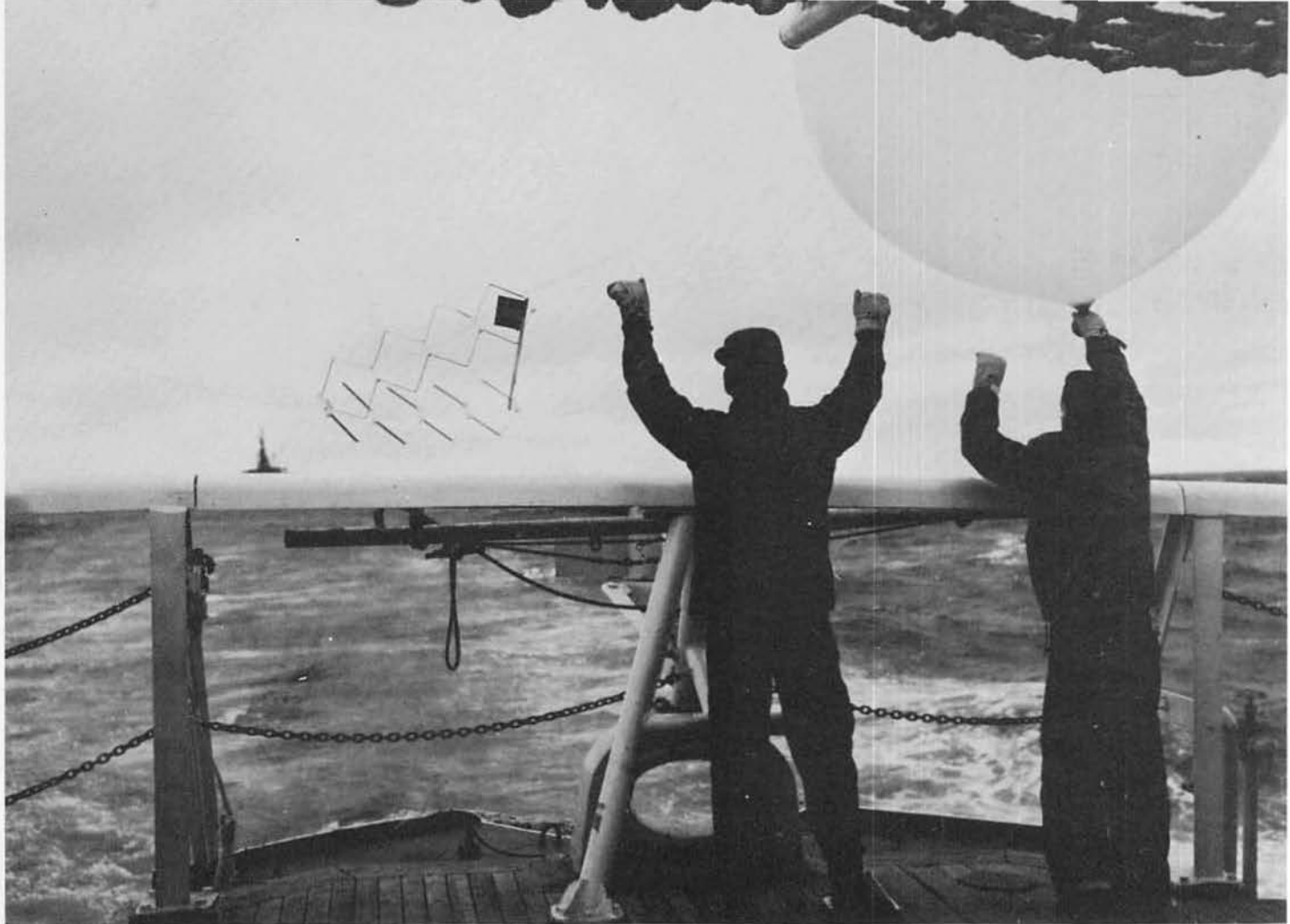
NAVAL AEROGRAPHERS RELEASE RADIOSONDE BALLOON; BOXED RADIO TRANSMITTER IS TOSSED.
