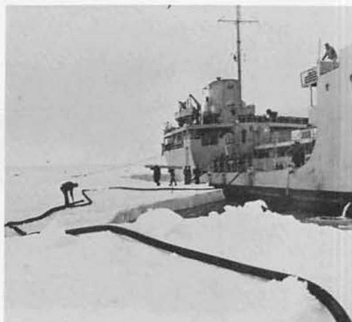
NESPELEN offloads avgas. Oiler is moored to ice by deadmen (far top). Fuel line is passed from ship to shore where it is hitched to 250,000-gallon storage tanks (at LAS and
