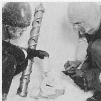
CORES ARE SAWN INTO SAMPLES, MARKED, WEIGHED.
