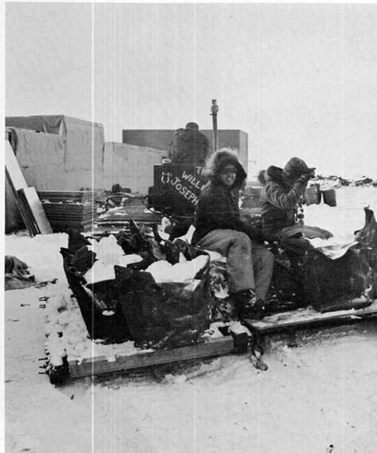
PARACHUTE bags full of snow for melter delivered at the station aboard tractor-drawn sled. This was before snow mine.
