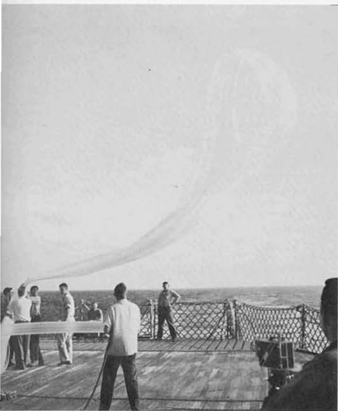
← ROCKOON launching: helium-inflated plastic balloon takes shape, rises; gas is pumped in until balloon reaches maximum height. Rocket attached is borne to 80,000 feet where it is launched still higher by remote control, radios back atmospheric data from space.
