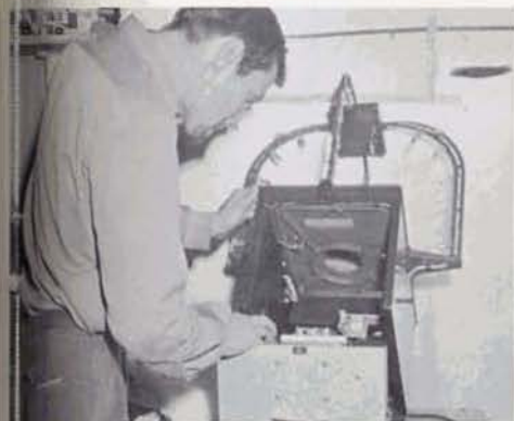
ALL-SKY CAMERA photographed 360 degrees of horizon, was automatically put in action by light or aurora.
