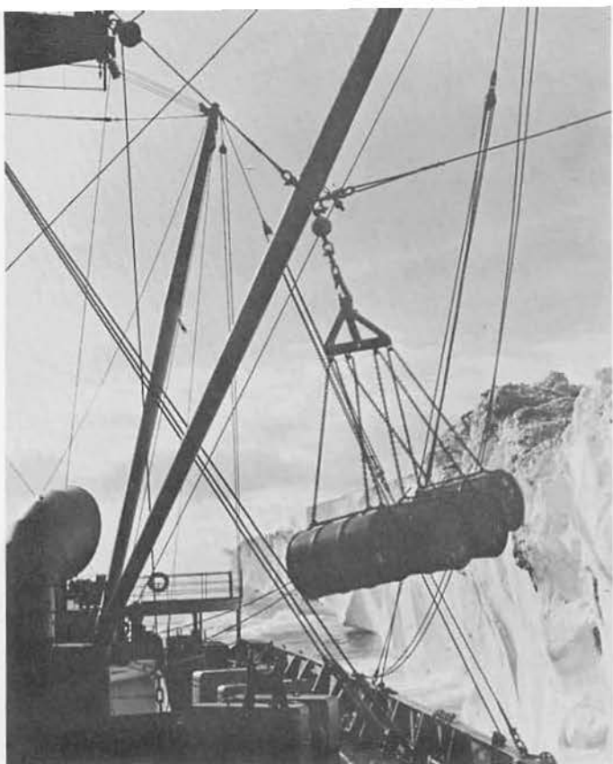
DRUMMED DIESEL FUEL OFFLOADED TO BARRIER.
