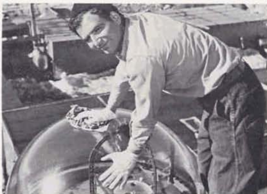
ALL-SKY CAMERA photographed 360 degrees of horizon, was automatically put in action by light or aurora.
