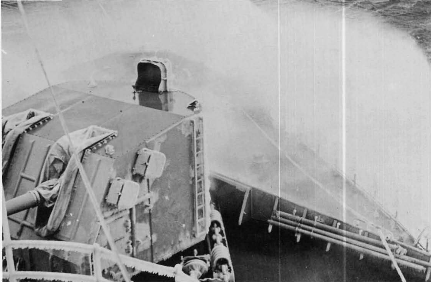
MOVING SOUTH, GLACIER BEGINS TO PILE ON ICE; BLOCK AND BRASH ICE LATER REDUCED SHIP'S ROLL.
