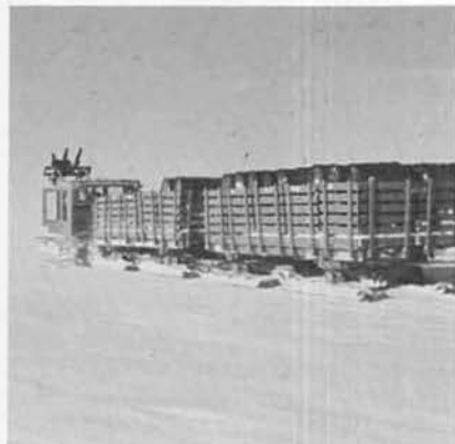
TRAIL and traverse parties received fuel and lube oil in drums by overland tractor-drawn sleds (Wilkes' S-2 ice-cap base) or by air delivery (Ellsworth traverse party).
