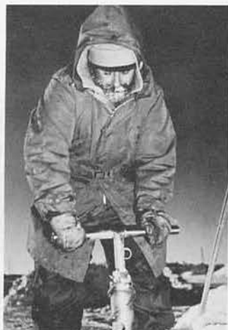
← IGY scientists Walter Boyd and Peter Shoeck test the density of snow with ramsonde equipment (left) as Al Crary drills for core samples of the vast ice shelf. Crevassed areas were source of data on stratigraphy.
