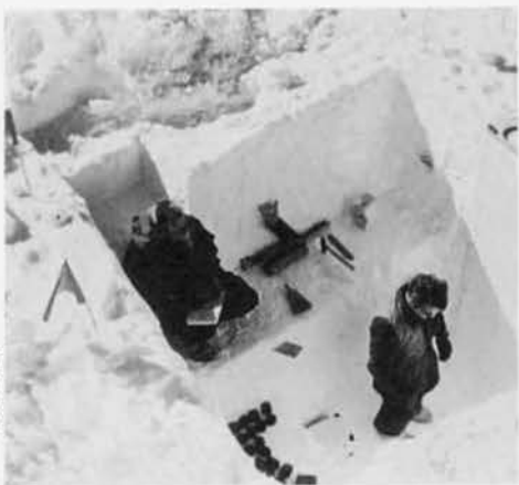
SHALLOW PIT on Byrd traverse was three meters deep (left). Ellsworth traverse party (right) stops to take snow samples from shallow pit dug in ice shelf.
