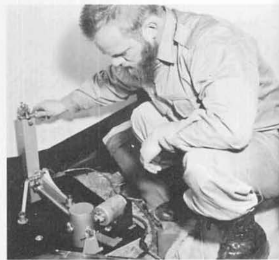
ologists (lower left) auger hole for seismic "shot." Station seismograph (directly above) records earthquakes for determining Antarctica's seismicity, for indicating average depth of icecap, for "previewing" formation of crevasses, for completing southern seismic network.
