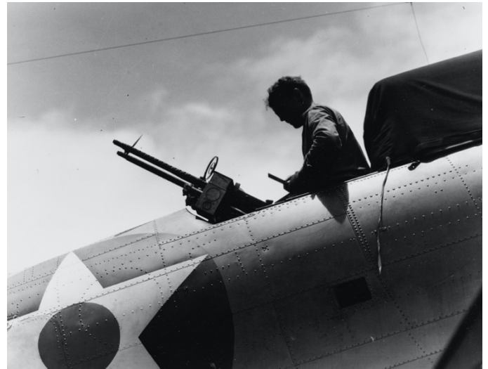
A crewman readies the rear cockpit twin .30-caliber machine-gun mount on a Douglas SBD-3 Dauntless onboard USS Enterprise (CV-6). Although this image was captured on 24 February 1942 prior to the launching of air strikes against Wake Island—more than three weeks after Bruno Gaido's exploit—it illustrates his "office" as an SBD radio-gunner well (80-G-66279)
