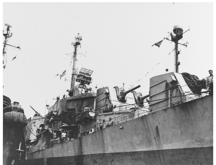
Comprehensive view of bomb damage on Laffey's starboard side abreast of her bridge (NH 75427).
