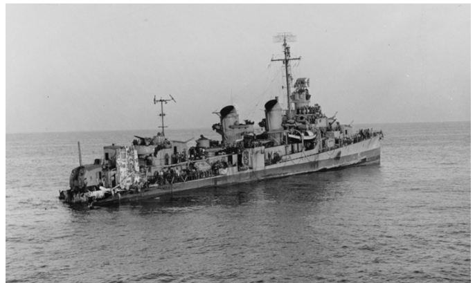
USS Sigsbee (DD-502), photographed from USS Miami (CL-89) after a kamikaze cut off her stern off Okinawa on 14 April 1945. She was towed to port and repaired (80-G-328579).
