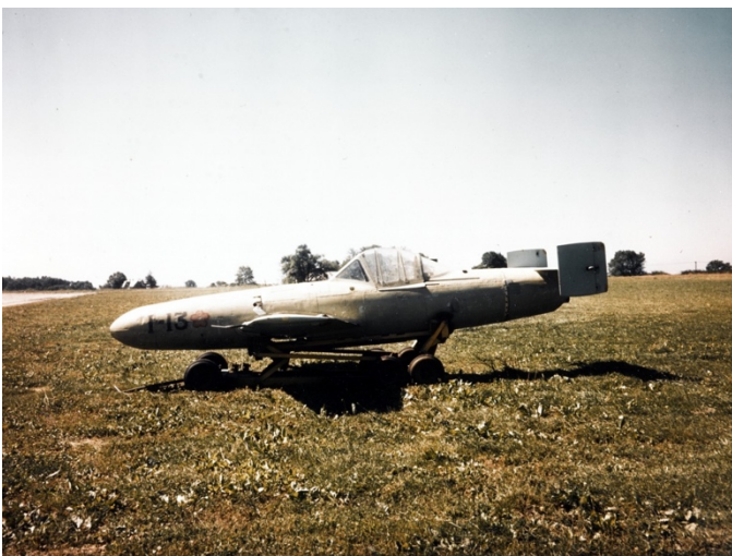
Japanese Yokosuka MXY7 Ohka ("Baka") piloted flying bomb captured intact by Marines on Okinawa. Photographed 26 June 1945 (80-G-K-5885).
