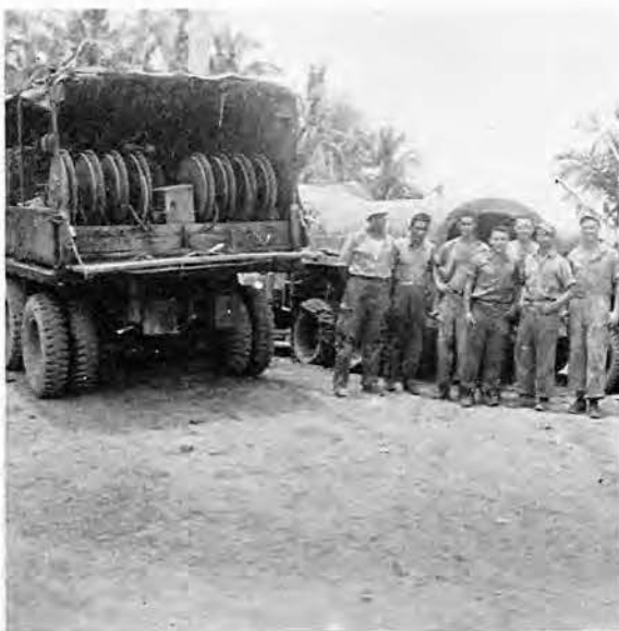
Equipment is fueled and greased in the field, by these mobile units
