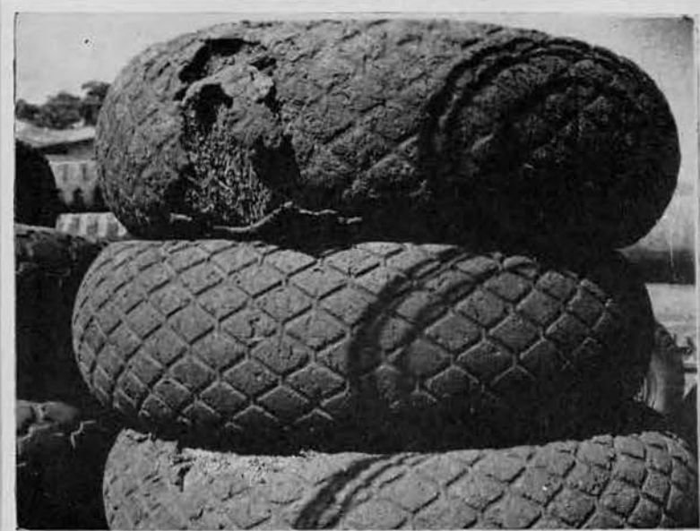
Right: Jagged coral terrain took a heavy toll of construction equipment tires.
