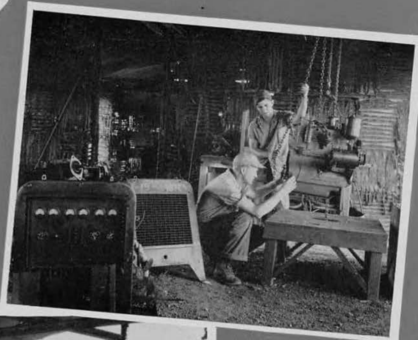
Portable generators are overhauled and checked regularly.
