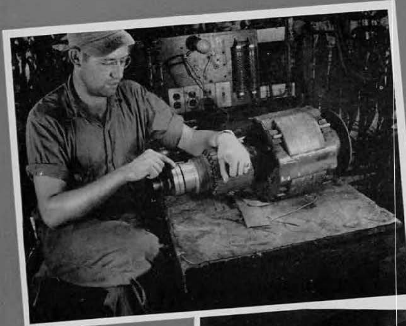
Rewinding and cleaning of an armature on a heavy generator.
