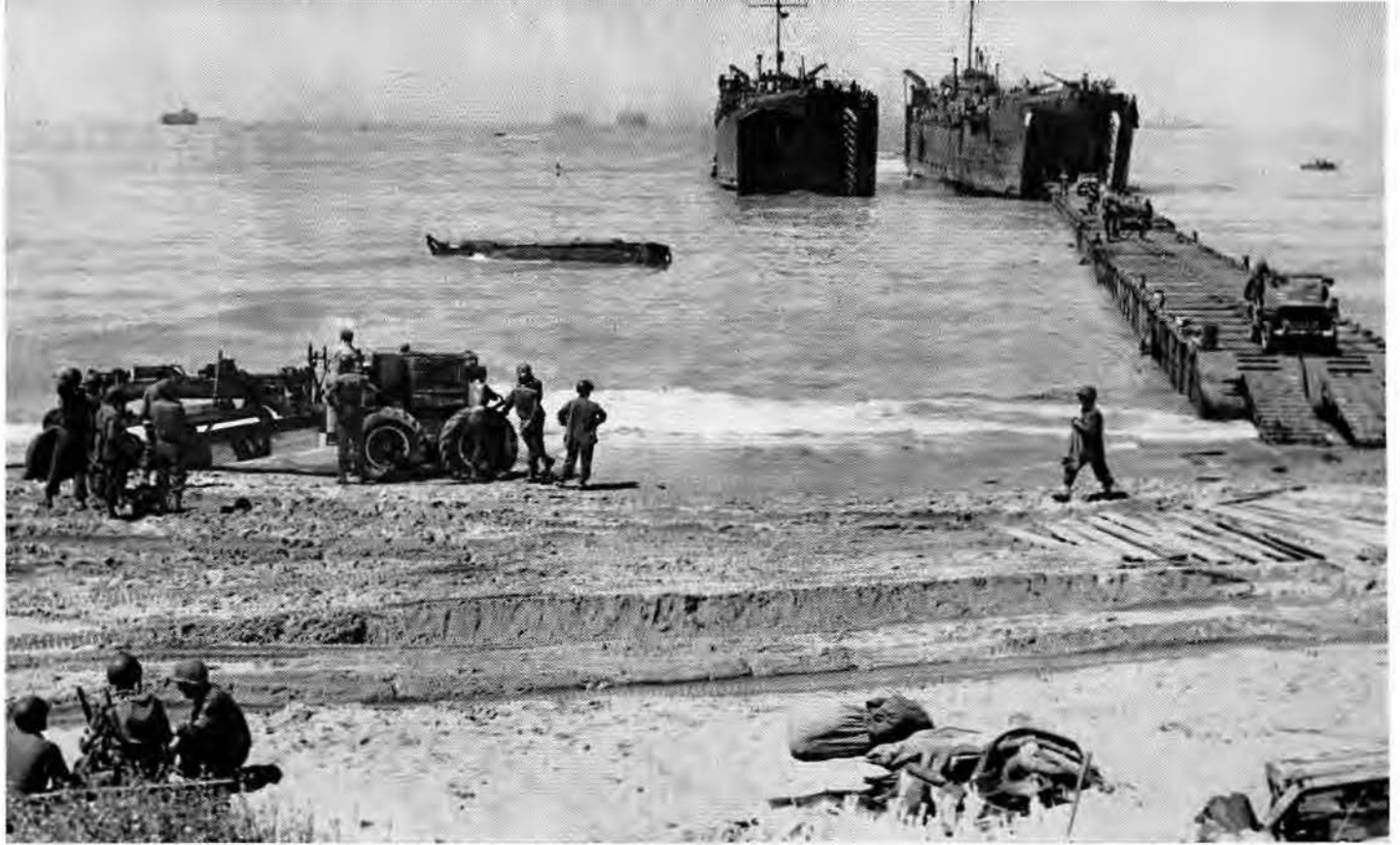
Bringing the war to the Italians, LSTs formed a large part of the huge armada that landed men and supplies on the shores of Sicily. Jeeps roll from one craft as another stands by, jaws open, ready to unload. Notice the pontoon causeway over which the jeep comes ashore.
