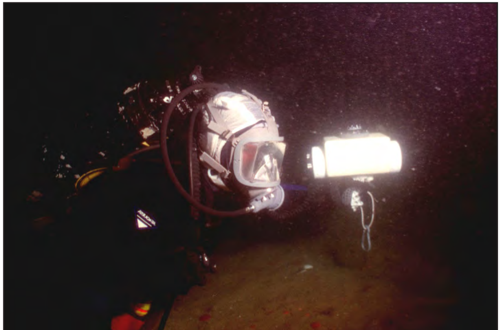
Figure 6-3. Explosive Ordnance Disposal Diving. An EOD diver using handheld sonar to locate objects underwater.
