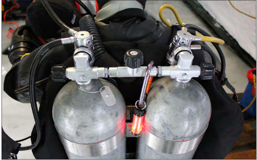
Figure 11-1. Two SCUBA cylinders fitted with two actual redundant first-stage regulators with GLO-TOOB attached.
