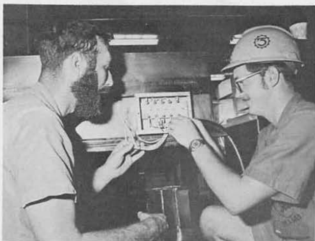
CE2 Gene St. Louis, Roseville, Minn., and CE3 Bob "Booby" Steil, Arroyo Grande, Ca., rewire the galley grill.
