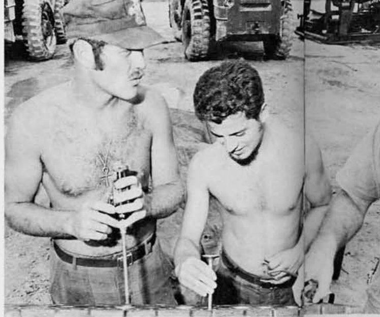
CM3 Mark Smith, Aurora, Neb. and CMCA William "Hernando Revolver" Sandoval reseat TD-20 head valves.
