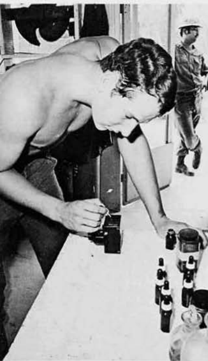
UTCN Dave Keller, Seattle, Wash., checks the chlorine content of fresh water at the water point.
