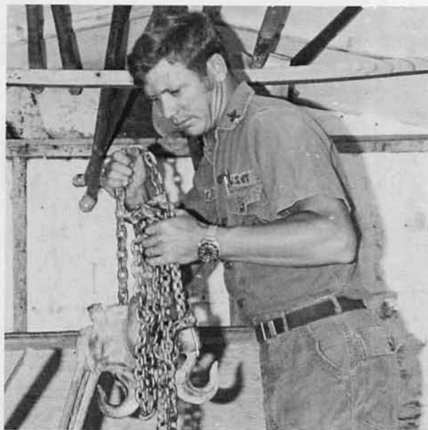
UT2 Nicky Dordon sets a up chain hoist in the UT trailer.
