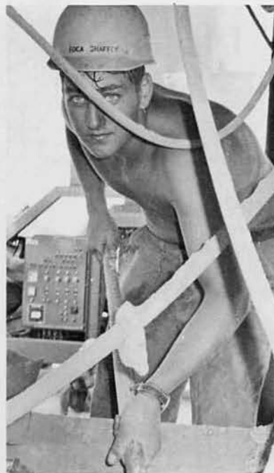
EOCA John Shaffer, Delmont, Pa., cleans the pug mill, where asphalt, aggregate and fines are mixed for a final product.
