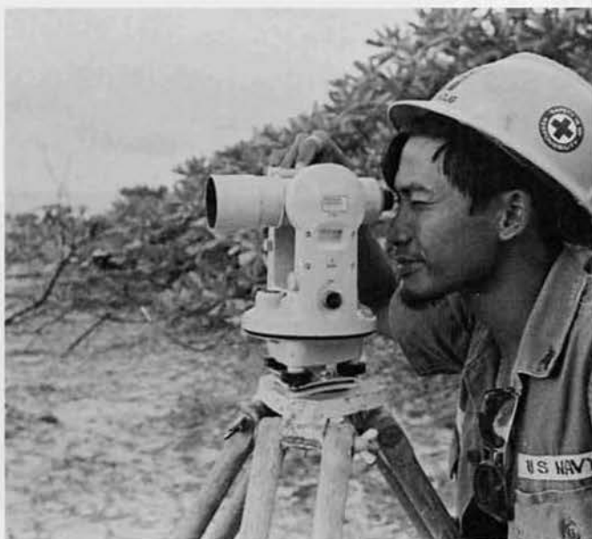
EA2 Ron Baclig on the transit, which is the basic surveying tool for the EAs.
