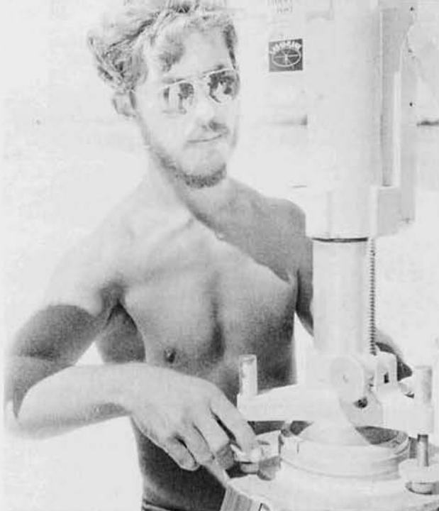
EA3 Ron Warner, Spring Valley, Ca., levels the laser plane, which simplifies surveying chores by eliminating the instrument man.
