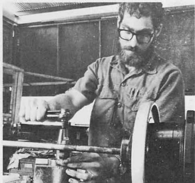
MR3 Frank Hayes, Flint, Mich., works on round stock on the metal lathe in the MR shop.
