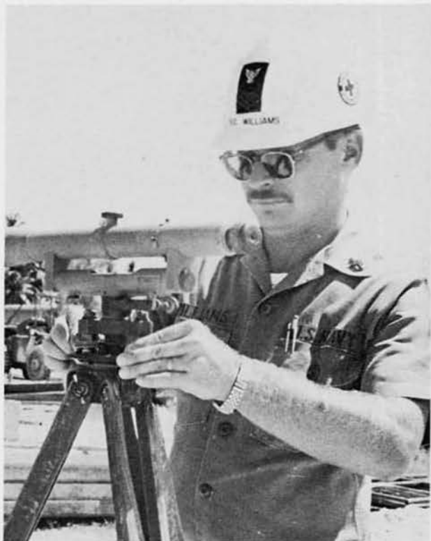
BUC James Williams, Grandview, Mo., levels a transit at the sub building.
