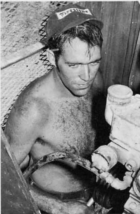
CMCN Tony Guenther, Oceanside, Calif., turns the crankshaft in an MRS over so CM3 Glover can remove the bolts from the flex-disc which is attached to the torque converter on the Allison 4460-2 transmission. RIGHT: CM2 Lilio C. Balmes, a submariner, now proudly wears his dolphins on Seabee Greens.
