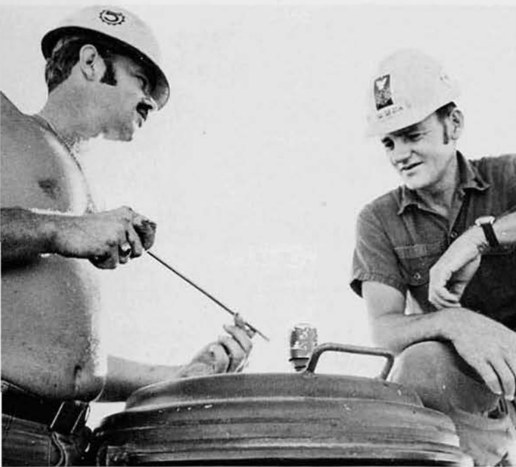
EO3 Vic Lovell and EO1 James J. "JayJay" Smith, Cascade, Ia., check out the hydraulic level on a 120 Hough front end loader. The 120 hydraulic system holds 55 gallons of fluid.
