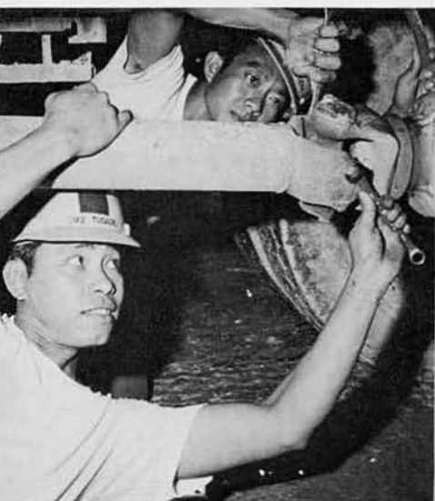
CM2 Tony Tugade and CM2 Apolonio Barcena remove the propeller shaft (i. e. drive shaft) from a 5-ton.
