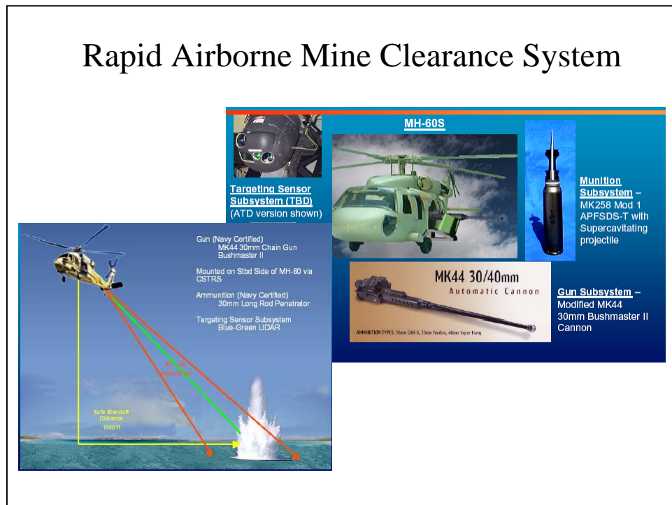
Figure VII-6 RAMICS Concept of Operations and Components
