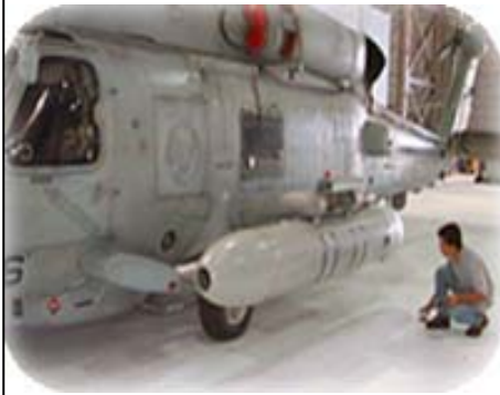
Prototype LASH system pod-mounted on SH-60.
