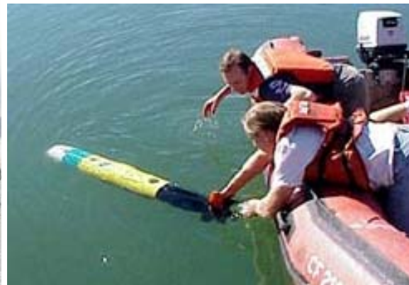
Figure 27 – Technicians Deploy a REMUS 100
