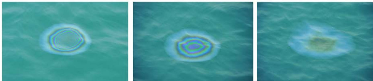
Figure 15. Three sequential images documenting a small oil seep over the DIVEX target as it rises to the surface of the water and disperses to form a small sheen.
