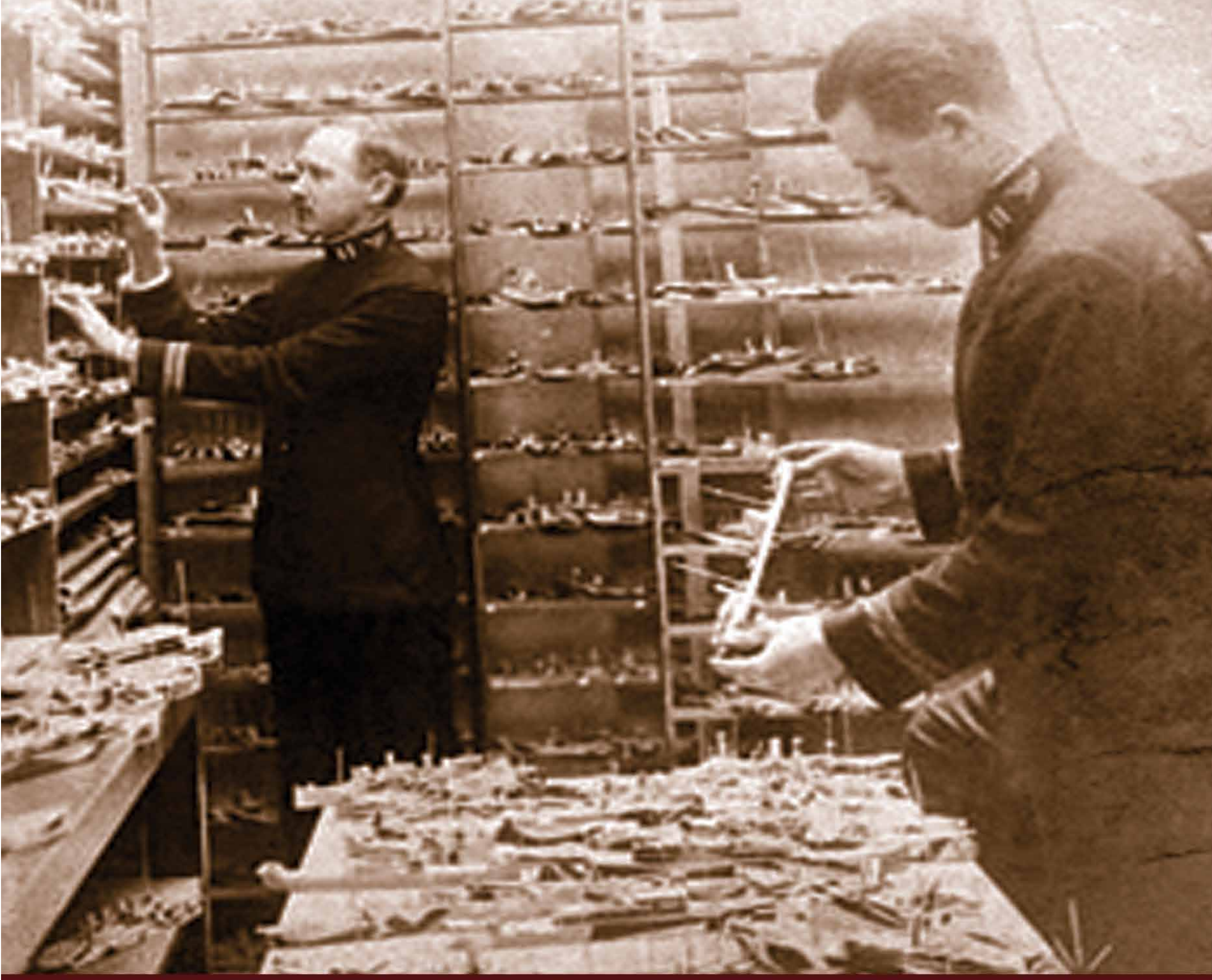
Jones' team developed an elaborate test theater that simulated the observation of ships in miniature. To recreate sea conditions, researchers viewed models from all aspects under varied lighting, through periscope-like optics.
