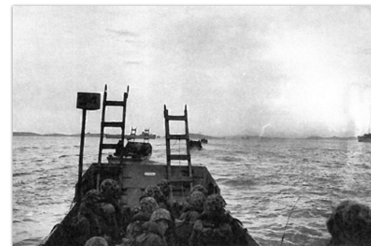
Navy LCVPs, loaded with Marines of the 5th Regiment, proceed in formation for the line of departure on the approach to Red Beach. The crudely built ladders standing erect in the bows of these craft enabled the Marines to scale the high sea walls barring their way to inland objectives. (NA W&C #1418)
