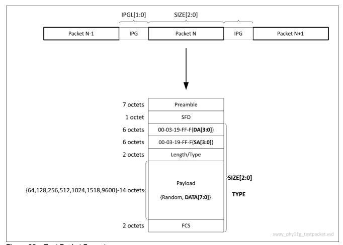
Figure 35 Test Packet Format
