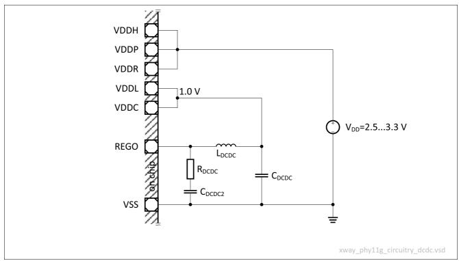
Figure 29 External Circuitry using the Integrated Switching Regulator
