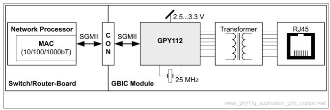
Figure 6 GPY112 Used in 10/100/1000BASE-T GBIC Application
