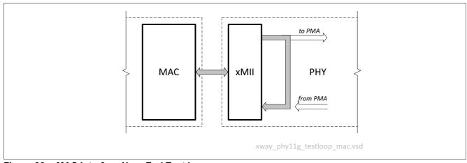
Figure 36 MAC Interface Near-End Test Loop
