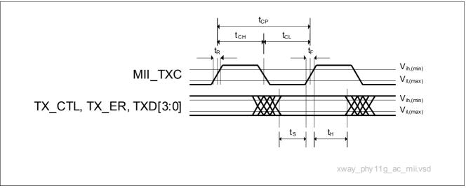
Figure 42 Transmit Timing Diagram of the MII
