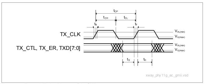
Figure 45 Transmit Timing Diagram of the GMII
