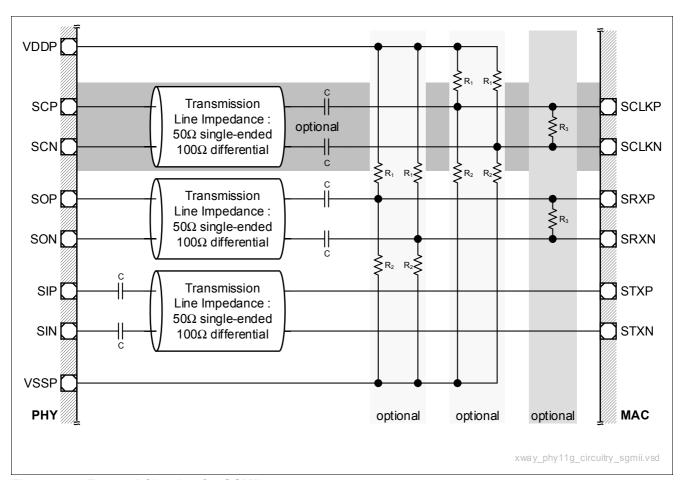
Figure 57 External Circuitry for SGMII
