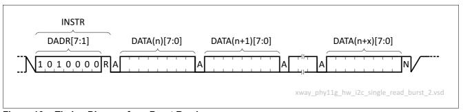
Figure 16 Timing Diagram for a Burst Read
