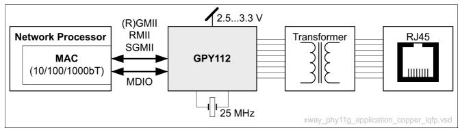
Figure 2 GPY112 Used in Copper Applications
