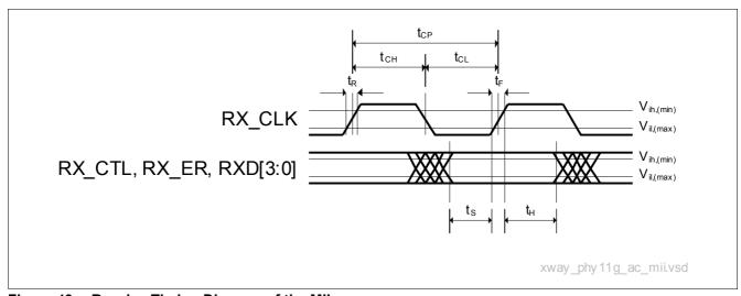
Figure 43 Receive Timing Diagram of the MII
