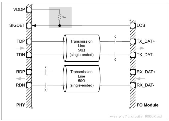
Figure 59 External Circuitry for a 1000BASE-X Interface
