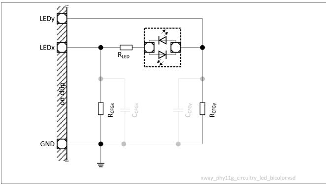
Figure 28 Bi-Color LED External Circuitry
