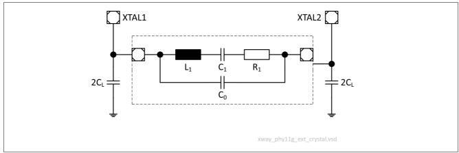
Figure 53 Equivalent Circuit for Crystal Specification
