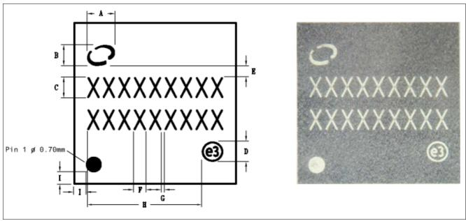
Figure 62 Chip Marking of PG-LQFP-64
