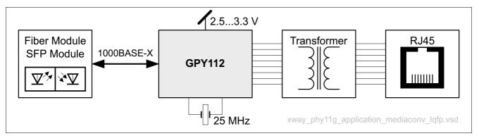
Figure 4 GPY112 Used in Media Converter Applications
