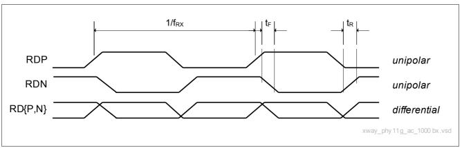
Figure 52 Receive Timing Diagram of the 1000BASE-X
