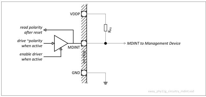
Figure 26 External Circuitry for an Active-Low MDINT
