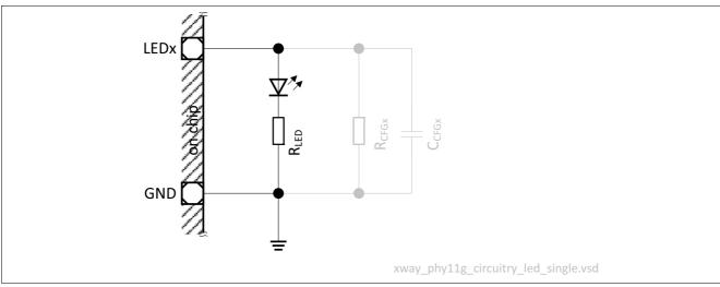
Figure 27 Single Color LED External Circuitry
