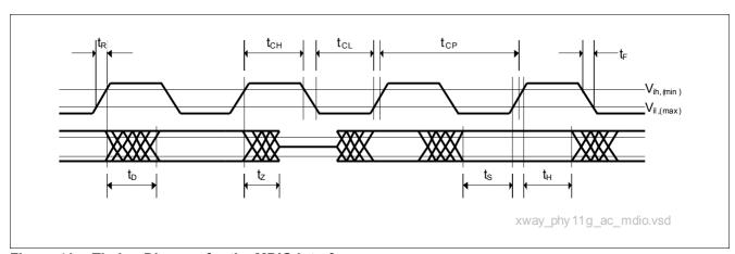
Figure 41 Timing Diagram for the MDIO Interface
