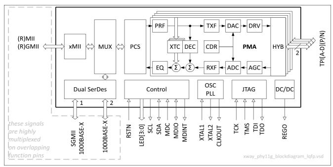
Figure 9 Functional High-Level Block Diagram of GPY112
