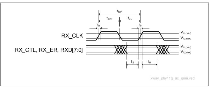
Figure 46 Receive Timing Diagram of the GMII
