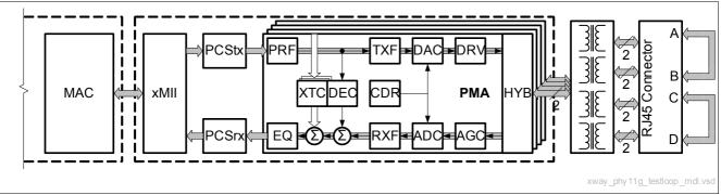
Figure 37 MDI connector Near-End Test Loop
