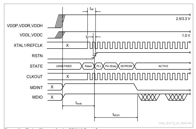
Figure 40 Timing Diagram for the GPY112 Reset Sequence
