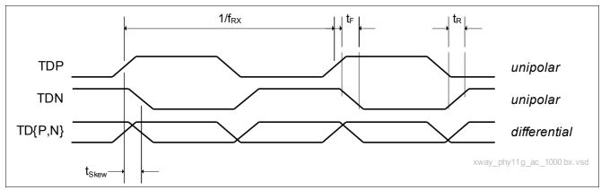
Figure 51 Transmit Timing Diagram of the 1000BASE-X Interface
