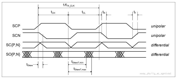
Figure 49 Transmit Timing Diagram of the SGMII
