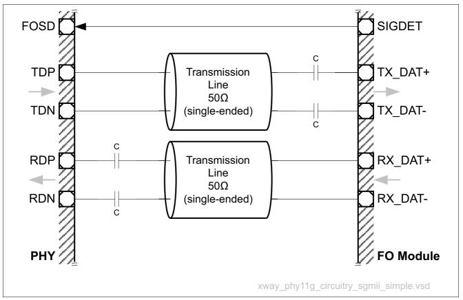
Figure 58 Simplified External Circuitry for SGMII
