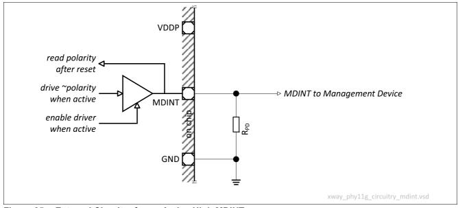
Figure 25 External Circuitry for an Active-High MDINT
