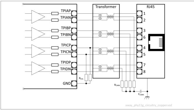
Figure 56 Twisted-Pair Common-Mode Rejection and Termination Circuitry
