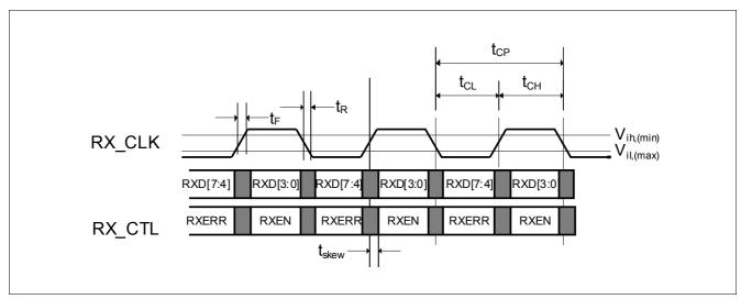
Figure 48 Receive Timing Diagram of the RGMII
