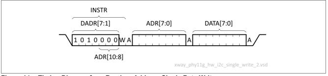
Figure 14 Timing Diagram for a Random Address Single Byte Write
