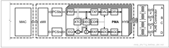
Figure 38 Echo Near-End Test Loop
