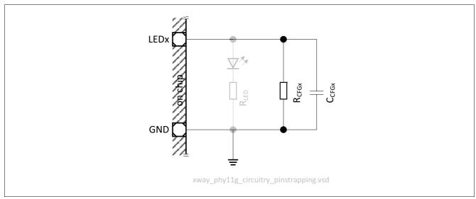
Figure 13 Soft Pin-Strapping External Circuitry
