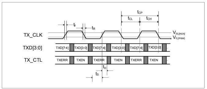
Figure 47 Transmit Timing Diagram of the RGMII
