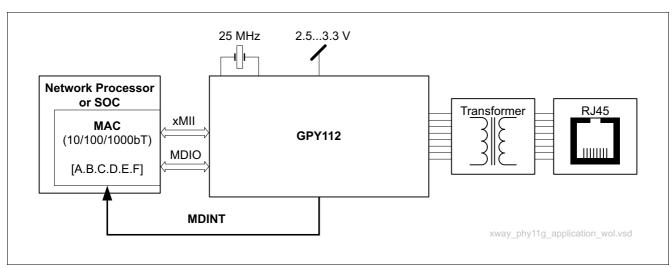
Figure 32 Block Diagram of a WoL Application
