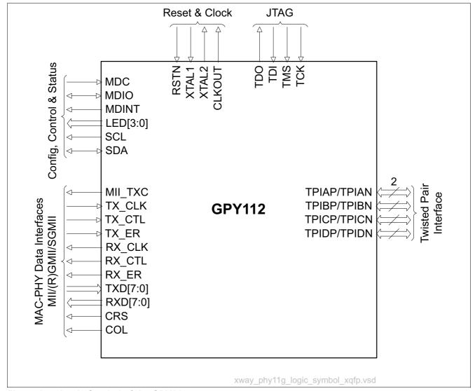
Figure 1 Logic Symbol of the GPY112
