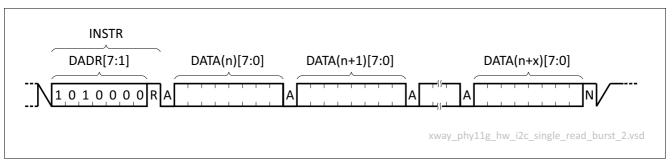
Figure 19 Timing Diagram for a Burst Read
