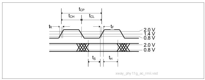
Figure 44 Transmit/Receive Timing Diagram of the RMII
