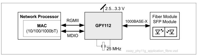
Figure 3 GPY112 Used in Fiber Applications
