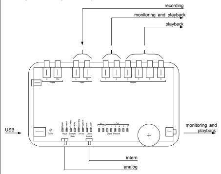
This is the set up for recording via the analog inputs while monitoring through the analog outputs. The clock source switch is set to *Intern*, the input selector to *Analog*. If you wish to take advantage of the EMI 2l6's latency-free monitoring, you should use outputs 1 and 2 or the headphone out.
