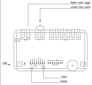
To use the EMI 216 for basic A/D conversion, simply connect an analog signal to the two inputs and feed the digital out to the digital device of your choice. Transmission of the signal from the analog inputs to the digital output is achieved via the EMI 2|6's built-in monitoring function.
