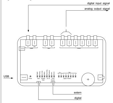
For D/A conversion, a digital signal is fed to the digital input and then passed to analog outputs 1 and 2 using the built-in monitoring function of the EMI 216. To avoid resampling, the EMI 216 should be synchronized to the incoming digital sig-
