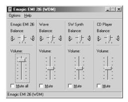
This illustration shows the volume control panel for the EMI 2l6. The playback level for audio recordings is controlled via the "Wave" slider. This control is placed *after* EMI 2l6's output. This means that EMI 2l6's master output fader in your music software can only control the full output dynamic range if both the "Wave" *and* the "Emagic EMI 2l6" sliders are set to maximum.
