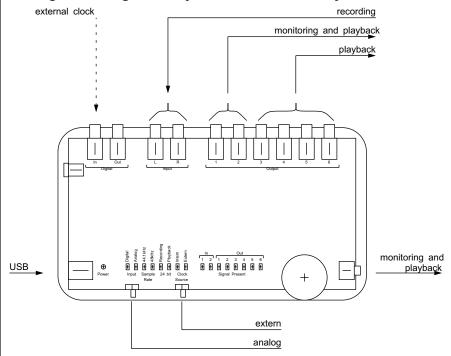
This set up is similar to "Analog Recording and Playback", as described above. Here, however, the EMI 216 is synchronized to a signal received at its digital input; the clock source setting is set to Extern. This setup is useful when the EMI 216 is used with another audio device with a digital output. By synchronizing the EMI 216 to this device, the sampling rates are locked to one an other which prevent long audio files from "drifting apart" during playback.
