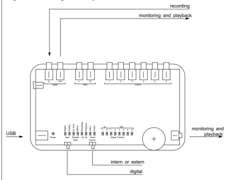
When recording from a digital source, the *Clock Source* setting is very important. The setting should correspond to the connected device—i.e. if a clock master device is connected, the switch should be set to *Extern*. If you insert an effects processor
