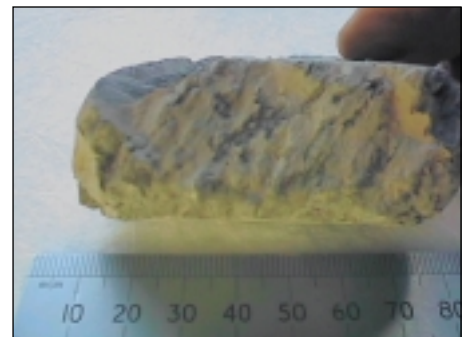
▲ Tabular caving (bottom) from natural fractures and angular caving (top) caused by breakouts. Scale is in mm.
