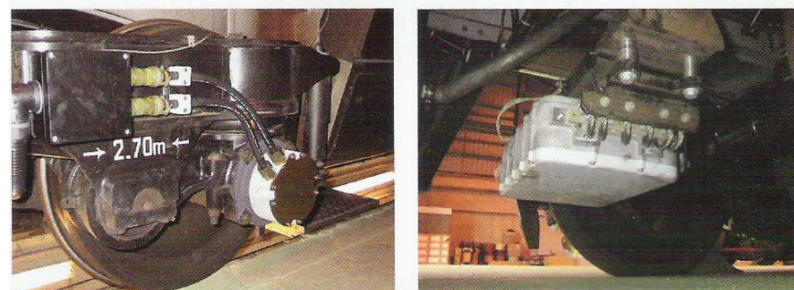
TASS Speed sensor (left) and bogie-mounted balise antenna (right) on a Pendolino train
