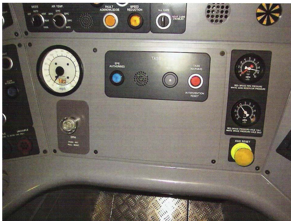
TASS Driver Machine Interface in a Pendolino Cab (Note: The Blue Lamp has since been renamed "Speed Supervised")
