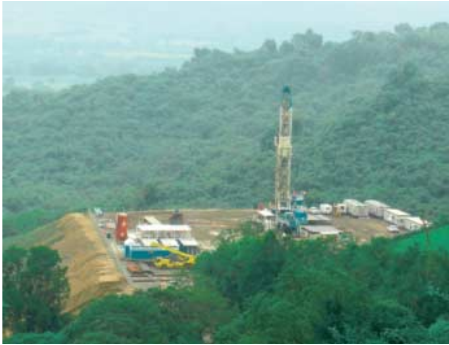
^ Chicontepec paleochannel drilling rig, built to optimize drilling times and logistics on multiwell pads in this environmentally sensitive area.
