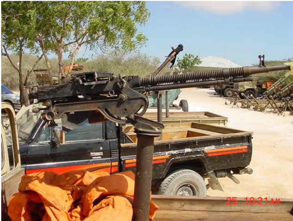
DSHK heavy machine gun mounted on a pick-up truck (other weapons in the background)
