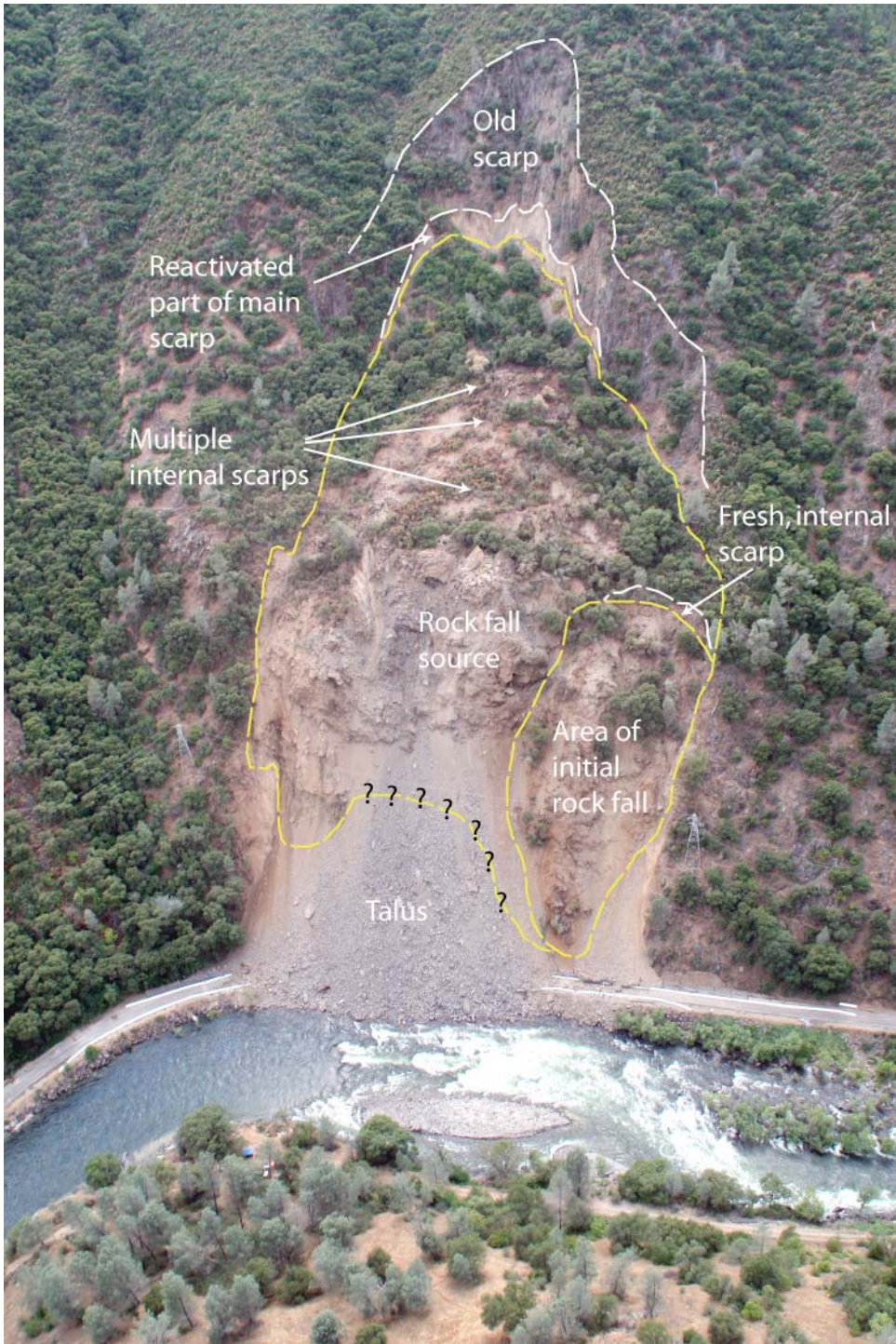
Figure 2. Oblique aerial photograph of Ferguson Rock Slide. Dashed yellow lines indicate extent of the rock slide based on visual inspection. Rock-fall source area, talus, and new scarps are indicated. Photo taken by Ed Harp on June 13 th , 2006.
