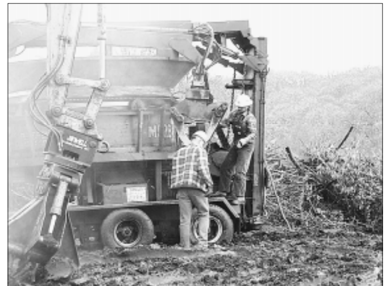
CHIP MAKING: Employees with Allwood Industries of Vancouver, Wash., prepe to grind wood debris into mulch that will be spread around trees and shrubs on campus. The university's wood recycling program has grown so fast in the past few years that Campus Recycling brings the wood grinder to campus twice a year.
