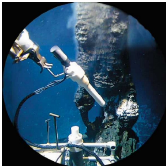
This chemical detector—the "electrochemical analyzer"—was built by scientists at the University of Delaware and Analytical Instrument Systems, Inc., in Flemington, New Jersey. It houses electrode sensors for taking chemical measurements at hydrothermal vents. The wand also is equipped with a thermometer. Image credit: University of Delaware Graduate College of Marine Studies.
