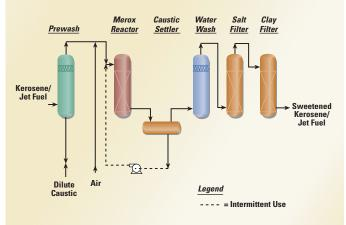
The kerosene leaving the caustic settler passes through a water wash which removes trace quantities of caustic as well as water soluble surfactants.
